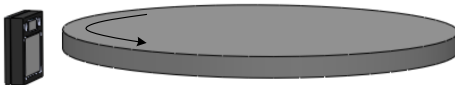
Figure 6. Tracking on a Disk Edge
