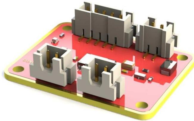
The TB6612 Motor Driver module is a low heat generation one and small packaged motor drive.
