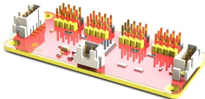
PCA9865 16-channel 12-bit I2C Bus PWM driver. It supports independent PWM output power and is easy to use 4-wire I2C port for connection in parallel, distinguished 3-color ports for PWM output.
