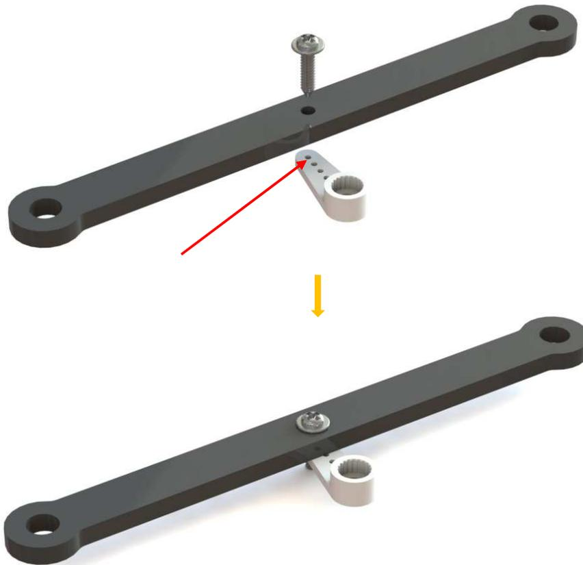
And also fasten them as tightly as possible, and then loosen the screw a little so the Steering Linkage can move flexibly.
