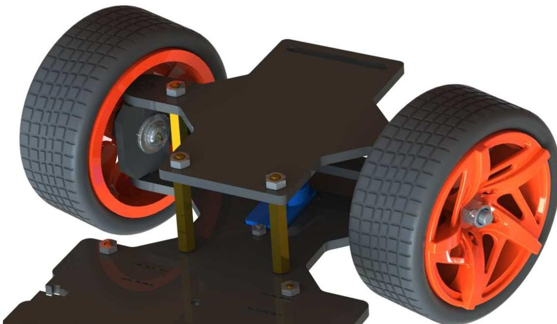
Hold them carefully, turn upside down, and fasten the standoffs and the Upper Plate with four **M3x8 screws**:
