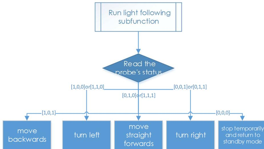
The light follower includes three phototransistors, thus its status list is composed of three elements which represent 8 statuses (based on permutation and combination). And here we need to set related responses to these statuses.
