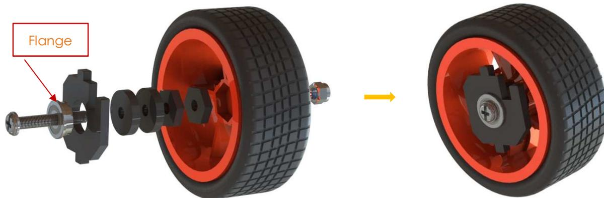
The Self-locking Nut should be screwed tight enough. It would be better to tighten the screw until the wheel and Steering Connector cannot move first, then loosen the screw a little, so that the Steering Plate can just move. Thus, the wheel can turn flexibly when the connection would not be too loose.
