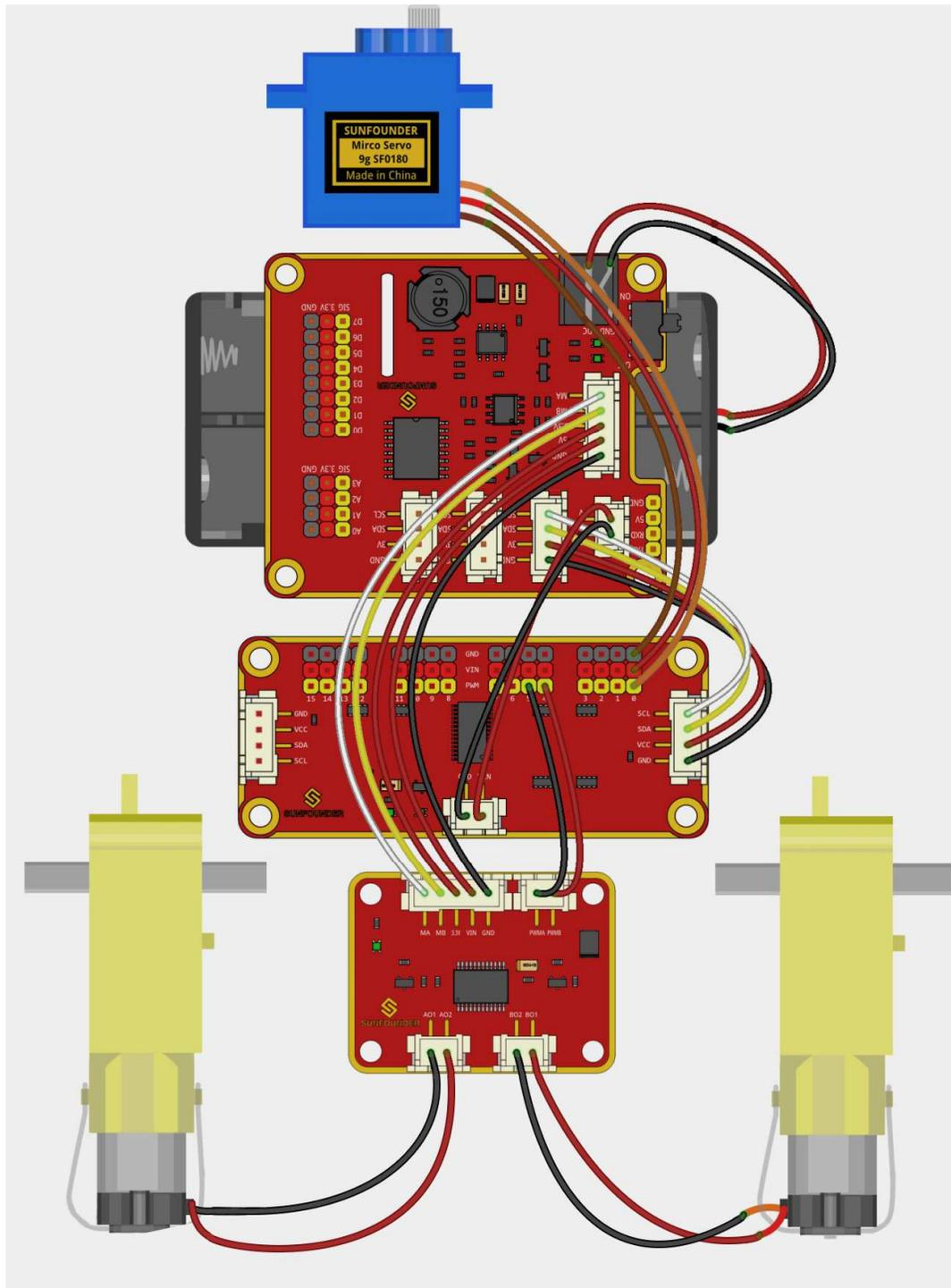
So now the circuit boards are all installed onto the car and the wiring is done. But still you're not ready to adjust the servo yet. First you need to complete some software installation.
