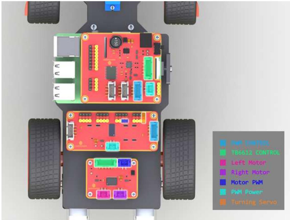
Connect the **PWM CONTROL** of the Robot HATS with the PCA9685 PWM Driver, and the **TB6612 CONTROL** with the TB6612 Motor Driver.
