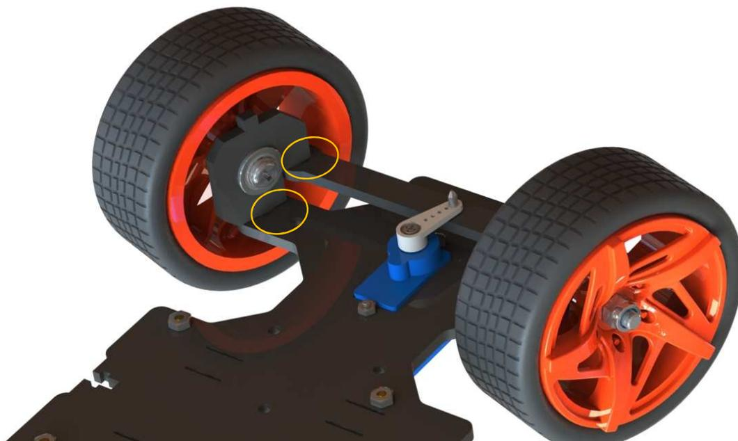
Then put the assembled Front Half Chassis onto the Upper Plate with standoffs aligned with the holes.
