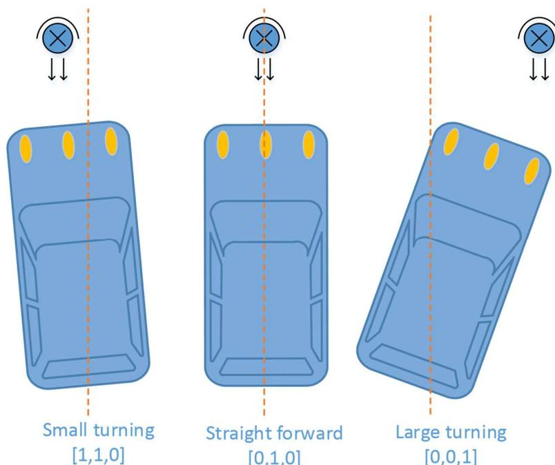
angle and small-angle turning. If the light is at the central left side (status `[1,1,0]`), we should apply a small-angle turning; if the light is at the edge of the left side (status `[1,0,0]`), we should apply a large-angle turning.
