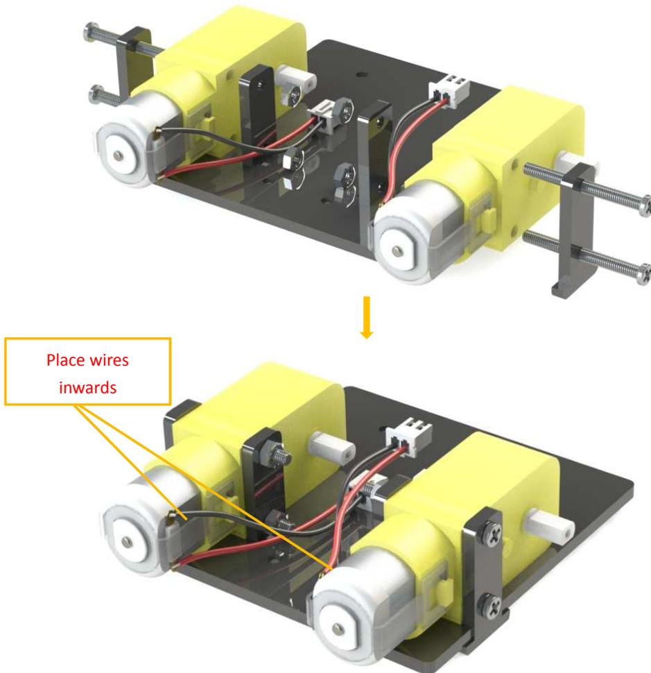
Insert four **M3x25 copper standoffs** through the acrylic plate into four **M3 nuts** as shown below:
