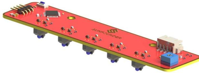
The TCRT5000 infrared photoelectric switch adopts a high transmit power infrared photodiode and a highly sensitive phototransistor. It works by applying the principle of objects' reflecting IR light – the light is emitted, then reflected, and sensed by the synchronous circuit. Then it determines whether there exists an object or not by the light intensity. It can easily identify black and white lines.
