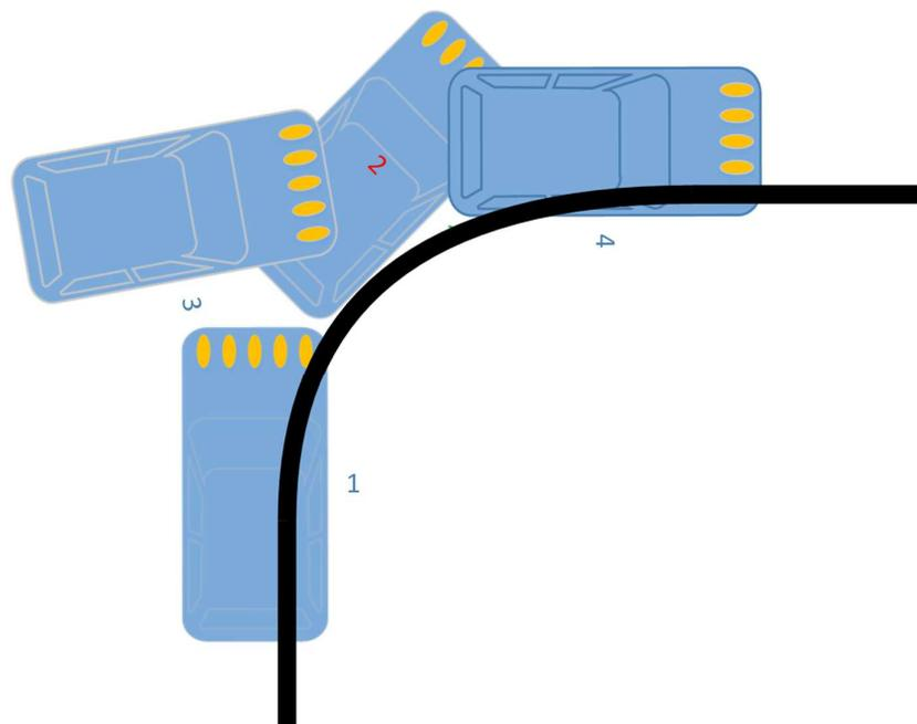
response program to let the car move backwards in the opposite direction (3), and then turn back to the original direction until a black line is detected again and move forward (4).
