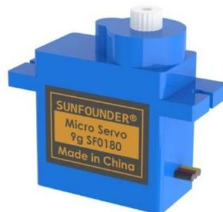
The SunFounder SF0180 Servo is a 180-degree three-wire digital servo. It utilizes PWM signal of 60Hz and has no physical limit – only control by internal software to 180 degrees at most.
