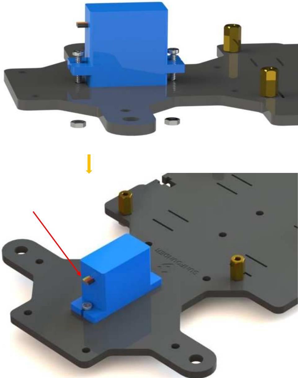
Till here the car assembly is mostly done. But **don't hurry** to assemble the front wheels, because the servo has not been adjusted yet. An unadjusted servo may get stuck and further get hot and burnt when it is connected to power to use as it is. To adjust, you can use your own way, like uploading an [Arduino program](#) to the servo which makes it rotate to the 90 degrees and stop, or using the [servo adjustment code](#) provided in this kit.
