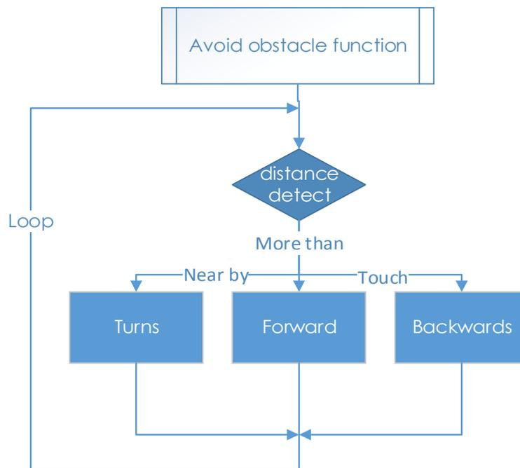
When the car starts, it will detect obstacles and measure the distance in cycle, make judgement, and take actions. Here are three cases: when the distance to the obstacle is  $x$  (the ranging distance threshold) away, the car will turn directions; when the distance is less than  $x$ , the car will move backwards before turning direction; when the distance is more than  $x$ , it will keep moving forwards.
