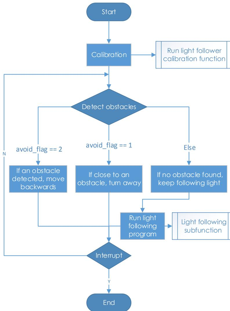
Since the light following and obstacle avoidance of the car depend on the sensor modules, we set two functions to read the status of two sensors separately, and assign values to flags to be returned from the functions: `state_light()`, and `state_sonic()`.
