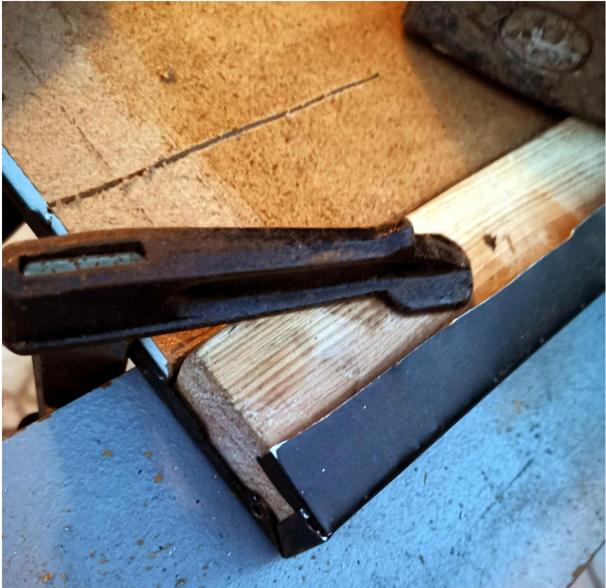
Using a piece of wood to avoid damaging the steel surface :
