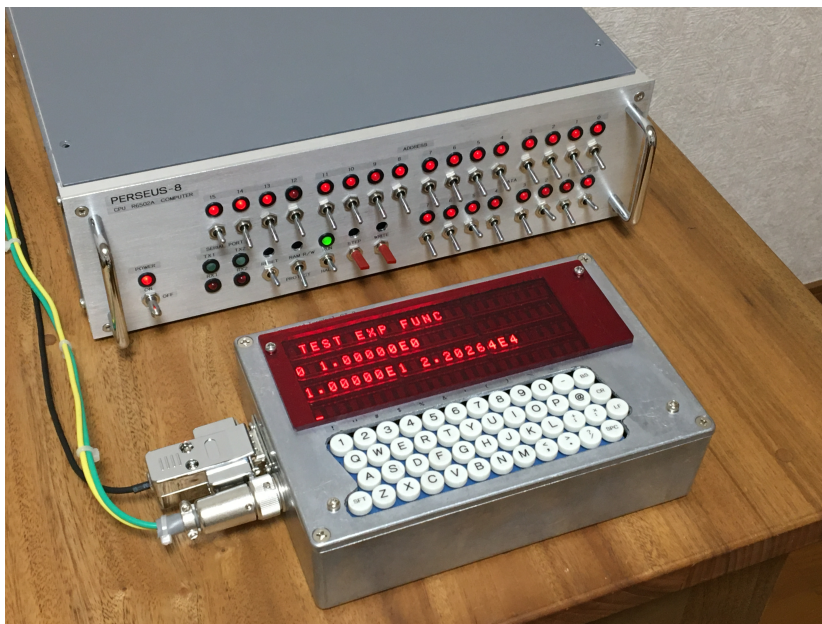
Fig.1 Floating point interpreter CI-2 running on my 6502 computer PERSEUS-8.
