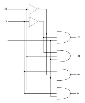
The AND gates are used as switches again. In this case, an AND gate can only be 'open' when a specific combination of bits is presented to the control inputs (00, 01, 10, or 11). In order to do this, each control input is also inverted.
