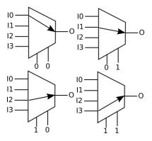
There are different MUX's possible with a different amount of inputs and control inputs. The most simple MUX only has one control input and two data-inputs. Its symbol would be:
