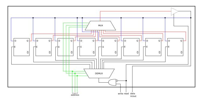
If the processor wants to write a bit in a certain location, the bit is presented at the 'data in/out' pin. The address is put on the address bus. The processor will then put the 'write' signal to 1 and the 'read' signal to 0. Now the enable signal of the selected D-latch is activated and allows the bit to be stored.
