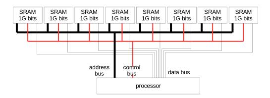
Each of the 'SRAM 1G bits' blocks is the same circuit as above, but with 1073741824 D-latches! The address bus is 30 bits wide in this case. The left SRAM will store all the MSB's of each location and the right SRAM will store the LSB's of each byte. On older computers one can see exactly this setup as there were 8 different chips on the memory modules. These days even more SRAMs are combined to the computer can read or write 64 bits in one go (the data bus is 64 bits wide is this case).
