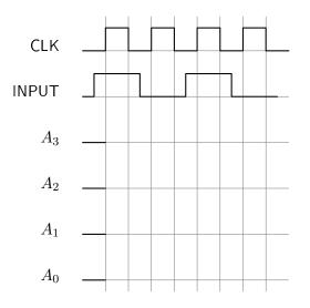
The INPUT signal is the serial data. The LSB is sent first and shifted all the way to the last flip-flop. After 4 clock cycles the data can be read in parallel from the outputs of the flip-flops.
