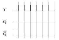
As you can see, the output of the T flip-flop is again a clock signal, but its frequency is divided by 2. This is how T flip-flops are often used: to divide a clock frequency by a power of 2 (one can put multiple T flip-flops after each other).
