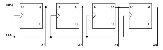
Every clock cycle (at the falling edge) all data in the register is shifted to the right and new data is read from the left. The following timing diagram shows the behaviour (complete it as an exercise):
