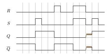
The top 2 rows show how the input is changed over time: R and S start at value 0, then S is put to 1 and back to 0. After this R is put to 1 and back to 0. At the end both R and S are put to 1 and released at the same time.
