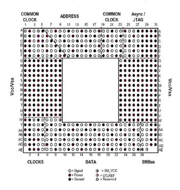
Here you can clearly see the pins for 'ADDRESS' and 'DATA'. In this case the address bus is 36 bits wide and the data bus is 64 bits wide. The processes can therefore read and write 8 bytes in one cycle. Can you determine the maximum RAM memory that can be accessed like this?
