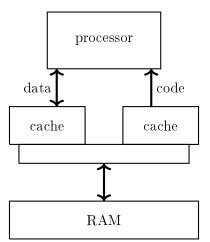
The cache memories are very small and are sometimes called 'level-2 cache' or 'L2 cache'. They contain a copy of a small portion of the RAM and they will refresh automatically when needed. The processor does not know this. It thinks it is connected to 2 RAM's. When the caches have to synchronise the processor is halted until the operation is done. This will still slow down the processor, but on average it will be faster than the Von Neumann alternative.
