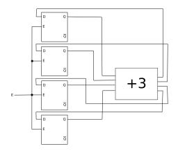
Clearly this cannot work. When E becomes 1 the latches will read and store the new number, but the output will immediatly be sent to the adder, therefore changing the input of the latches again. This results in erratic behaviour. There is no clock to synchronise the circuit.
