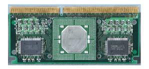
The two chips on the left and right are the caches for data and code. In modern processors these caches are integrated with the processor.
