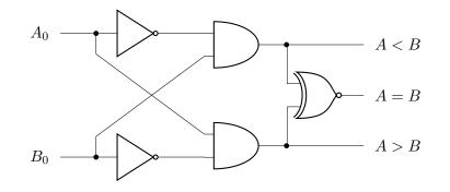
Remark that the output A=B is not calculated from the inputs. This is mostly done for aesthetic purposes (the lines do not cross), but it also illustrates a very important feature of the comparator: any output can be calculated from the two other outputs. This is because exactly one output is 1 at any time. This means the XNOR gate could also be replaced by a NOR gate which will output a 1 when the two other outputs are 0.
