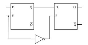
This combination is known as a 'master-slave D flip-flop' or simply a 'D flip-flop'. The second latch (the 'slave') will see the inverse of E. This means that when the first latch (the 'master') is 'closed', the second latch is 'open' and vice versa.
