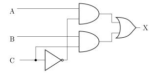
Remark that one can also intuitively understand the above circuit. The AND gates are used as switches. An AND gate can only output a one if both inputs are one. This means that if an input is zero, the AND gate cannot output a one. The AND gate is 'closed'. In the above circuit one input of each AND gate is connected to an input. The input can only travel through the AND gate if the other input is one. That is controlled by the control input.
