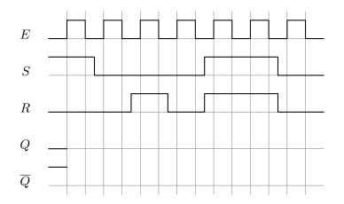
Remark that Q and  $\overline{Q}$  can only change while (and as long as) E = 1. When E = 0 the output will remain at the value that it had when E dropped to 0. The enable signal will let the input through, effectively storing the bit at the input.
