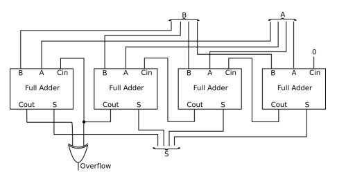
Four full adders are put in a cascade. The right most full adder adds the 2 least significant bits of A and B. Its carry-in is hard coded to 0. One could also use a half adder but being able to add 1 to the result by just altering that first carry-in has a lot of advantages (see e.g. exercise 5.6.5 at page 81).
