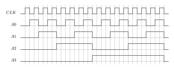
Every T flip-flop will divide its incoming frequency by 2 and give it to the next. If one looks at the output as one number (where A0 is the LSB and A3 is the MSB), the output evolves as follows at each falling edge: 0000, 0001, 0010, 0011, 0100, ..., 1111. After this the output will go back to 0000.
