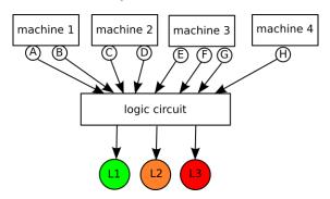
The output is determined by the 8 inputs. The truth table could look like the following:
