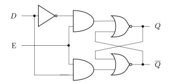
The input is now called 'D' (data) and presents a bit to be stored in the latch. The bit is only stored when E is equal to 1. While E is 1 the output will follow the value of the input D.
