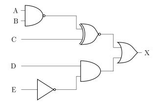
The operations are evaluated in the same order as in normal algebra: the AND operation has a higher precedence than the OR operation. XOR and OR are evaluated from left to right. Using brackets this order of evaluation can be altered or made more clear.
