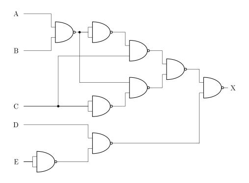
This is very important: one can build any logic circuit using only NAND gates! Implementing a NAND gate in any technology enables to create a complete computer.
