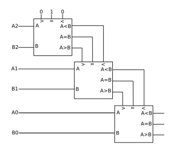
Each block is a comparator that compares 2 bits, but also takes into account the information of the previous comparison. There are now 5 inputs per comparator. But one can notice that one only needs 4 inputs because the fifth is determined by the other 4 (e.g. one can predict the = on the basis of < and >).
