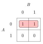
The input A is on the left side and the input B is on the top. They can both be 0 or 1 resulting in 4 squares in which the corresponding output is written. So the upper left corner corresponds to input 00, the upper right to 01, the lower left to 10 and the lower right to 11.
