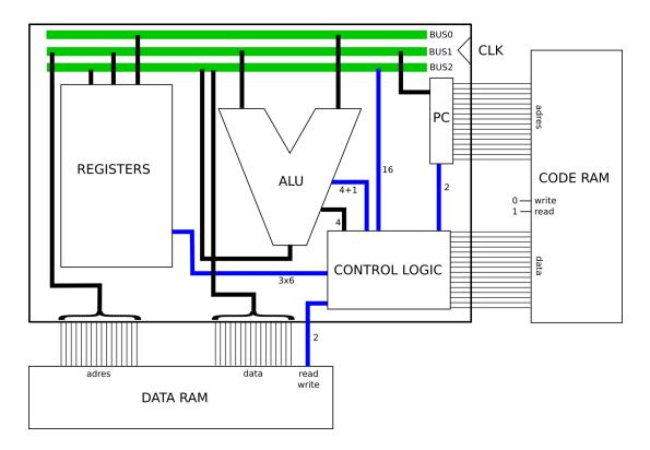
Two RAMs are connected to the processor. In this case both RAMs have an address bus that is 16 bits wide. The data bus is also 16 bits wide. A RAM can thus be regarded as an array of 65536 values. Each value is a 16 bit number.
