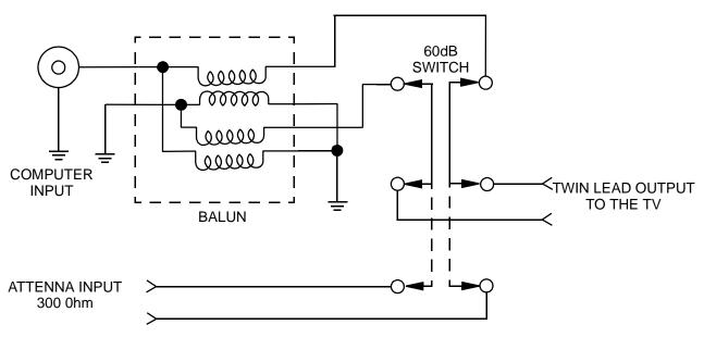
Figure 4. Antenna Switch Box Schematic
