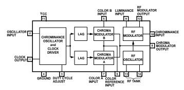
Figure 6. MC1372 Block Diagram
