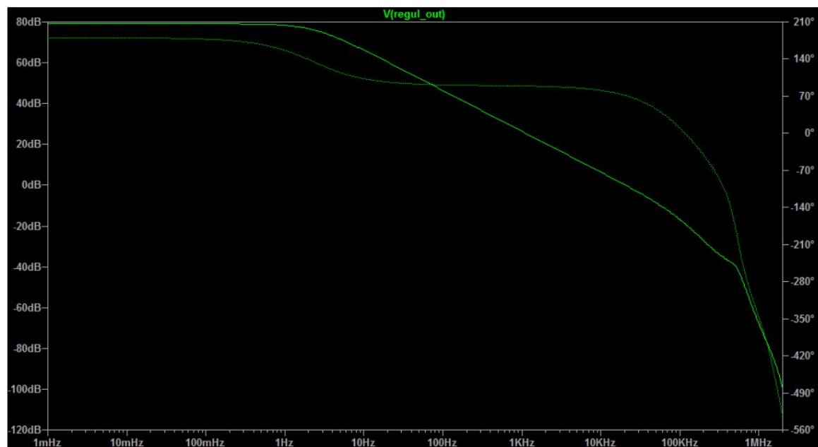
Graph 2: Transfer characteristic of the controller without a closed control loop
