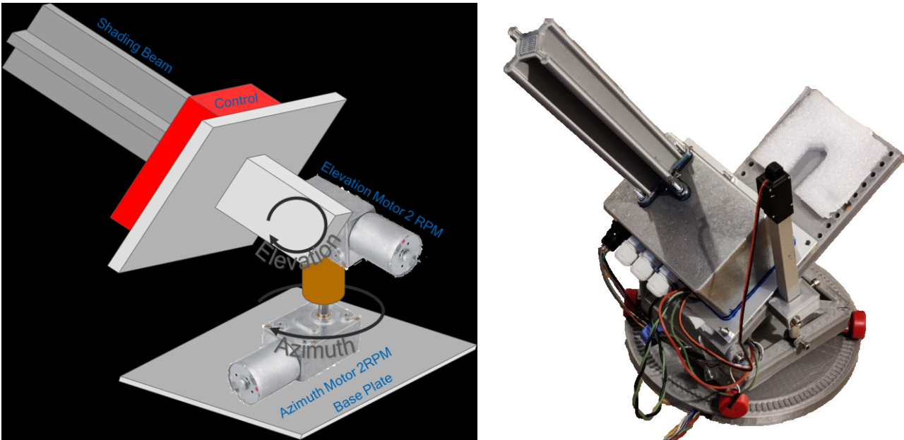
Fig. 2: Simple table top tracker and my table top tracker made from 3D-printed parts and Fischertechnik.
