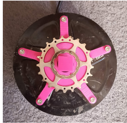
Fig. 14: Generator sprocket mounting mechanism.
