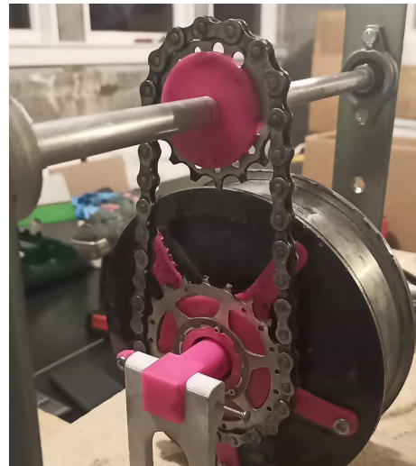
Fig. 15: Fully assembled gear train. Shaft running along the top is the driveshaft.
