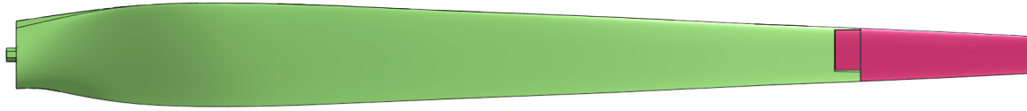
Fig. 8: Full span of blade, showing position of the segment joint (Interface between green and pink segments).
