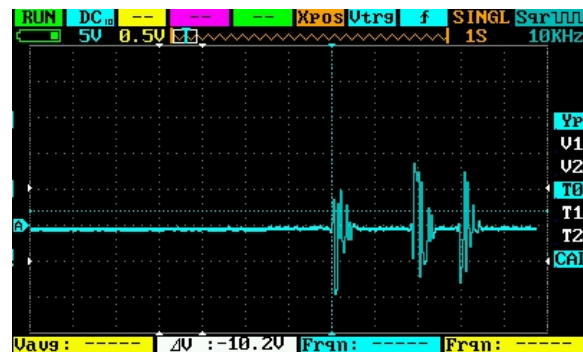
(a) Raw generator output. Pulses generated by manually rotating the generator as fast as achievable.
