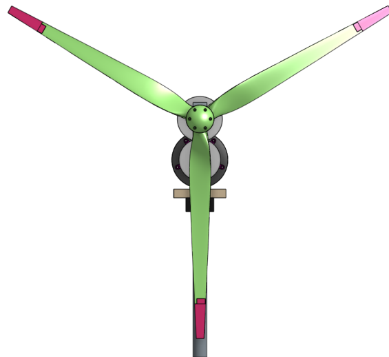
(a) Old SD7032 rotor design. Note the narrow root section.
