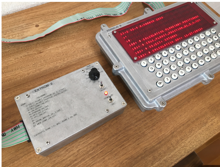
Fig. 5.2 Homemade PROM module EXTROM-2 connected to the parallel interface.
