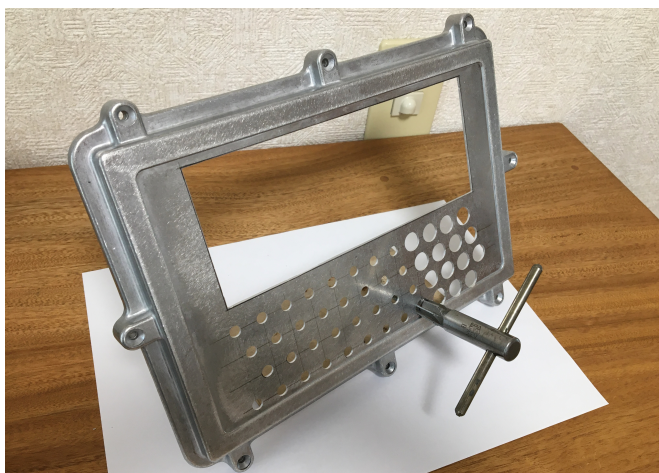
Fig. 3 Reaming work for enclosure.
