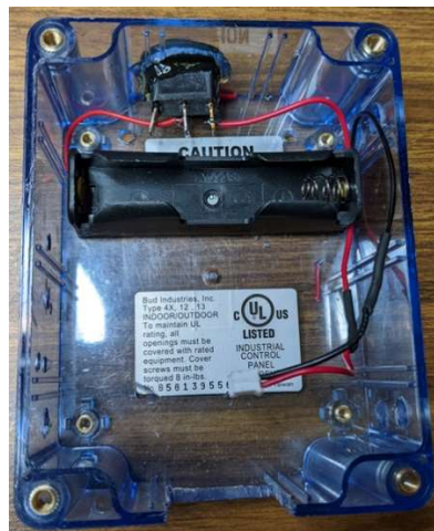
Figure 16. Enclosure with battery and power switch mounted
