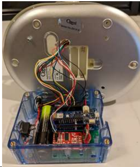
Figure 22. Attaching scale wires to electronics.
