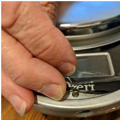
Figure 6. Access to top screw on scale cover
