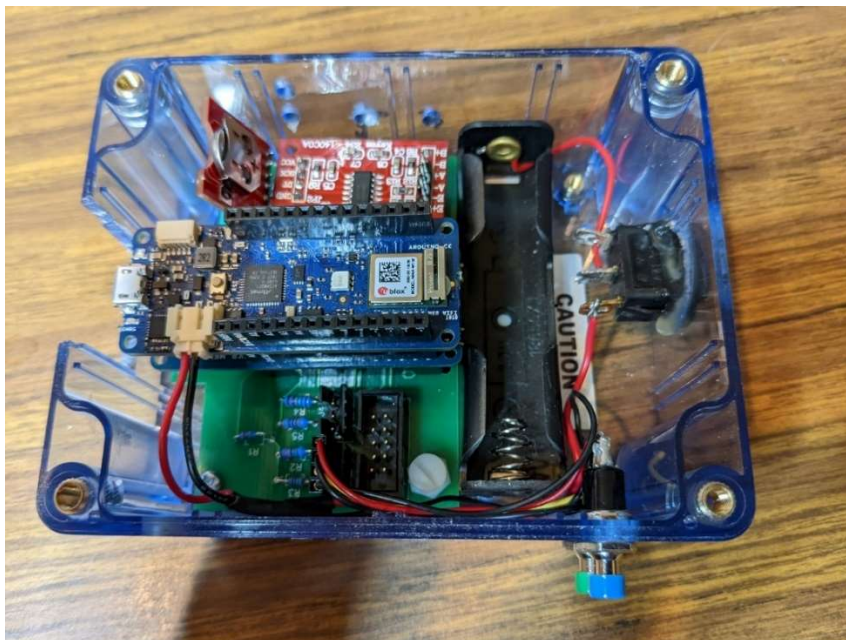
Figure 4. Mkr1010 system in enclosure
