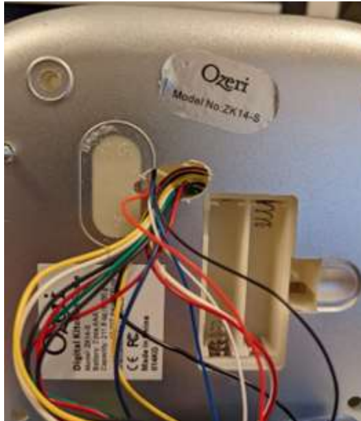
Figure 21. Slot on scale bottom for connections to electronics
