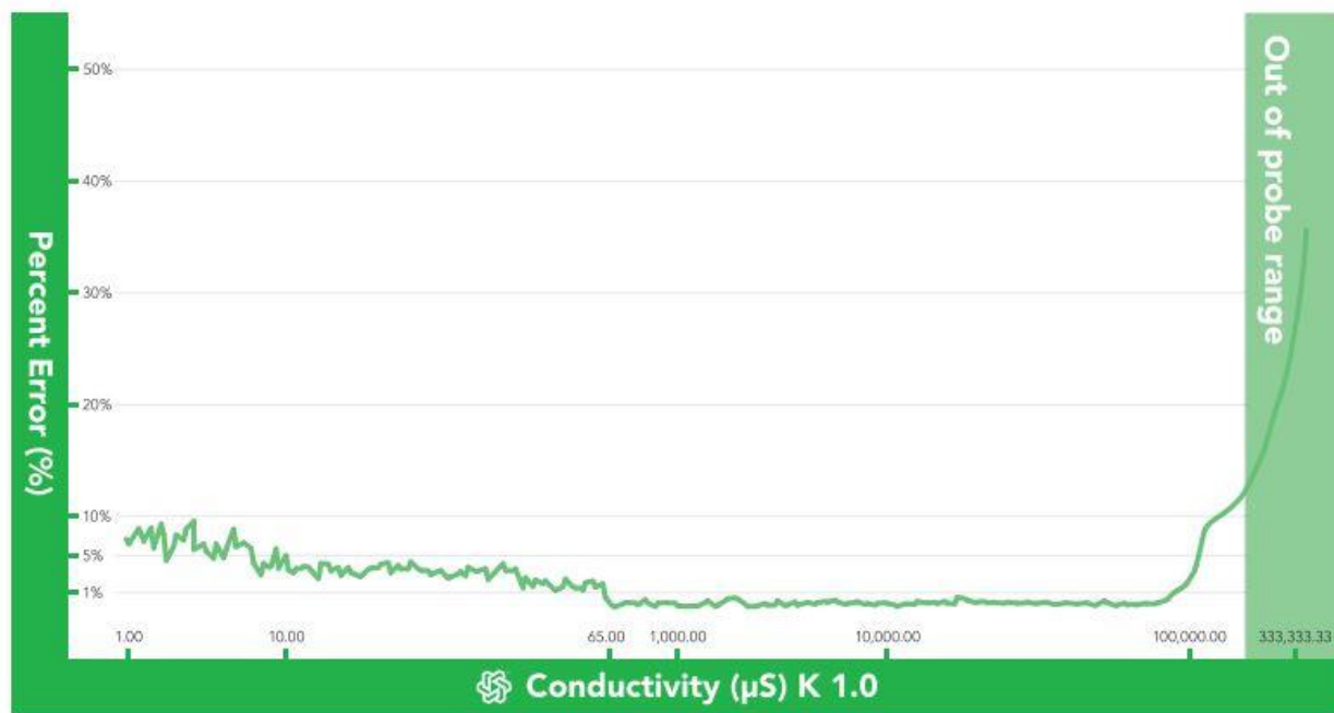
Figure 37. Accuracy of Atlas Scientific K 1.0 Conductivity Probe and EZO circuit. Data provided by Atlas Scientific.
