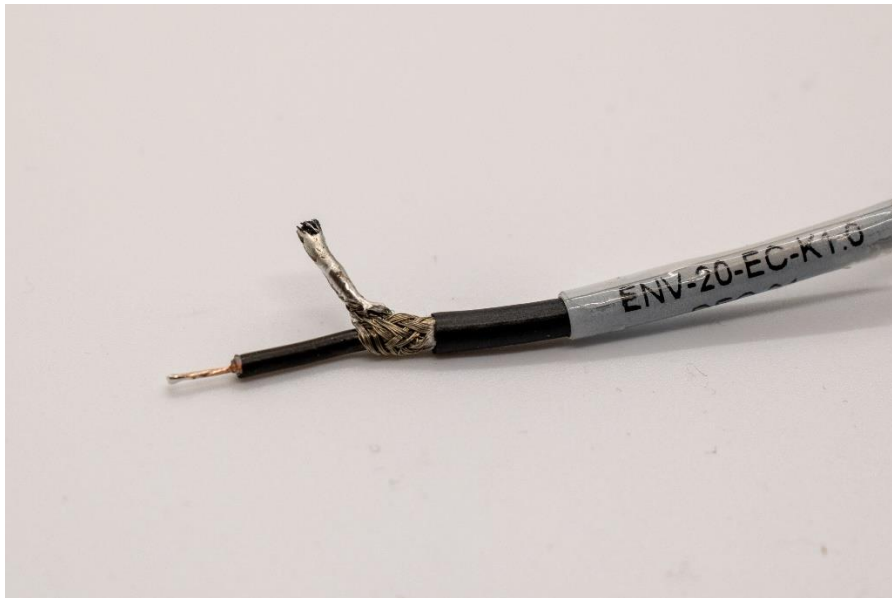
Figure 16. Conductivity probe leads with coaxial wires stripped and soldered.
