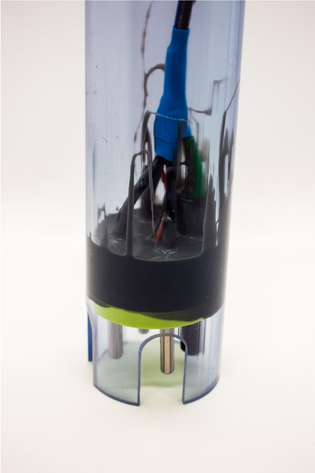
Figure 29. A clear OpenCTD showing the thick epoxy potting layer.
