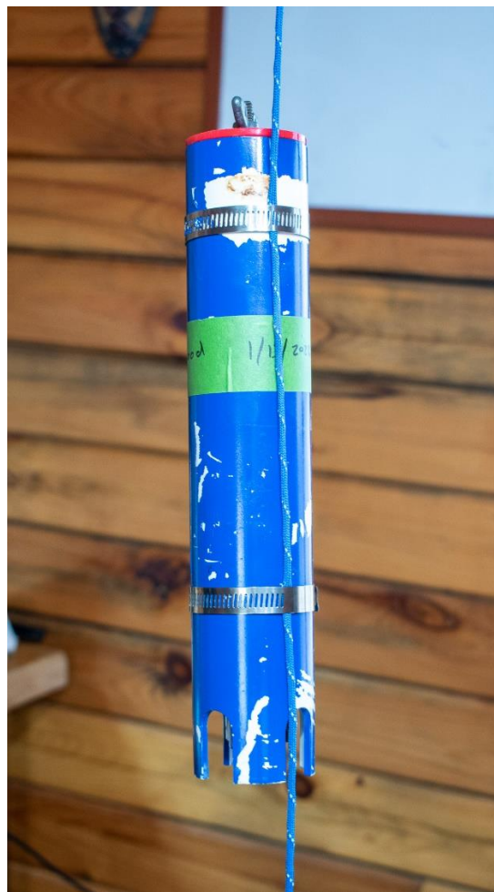
Figure 33. Example of OpenCTD attached to weighted anchor line using hose clamps.
