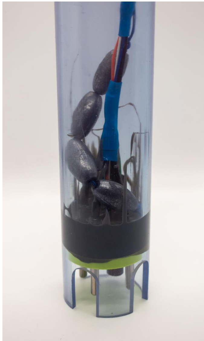
Figure 34. Clear OpenCTD with fishing weights inside.
