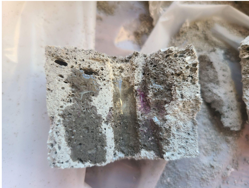
Fig 2: Treated sample tested with phenolphthalein shows complete carbonation
