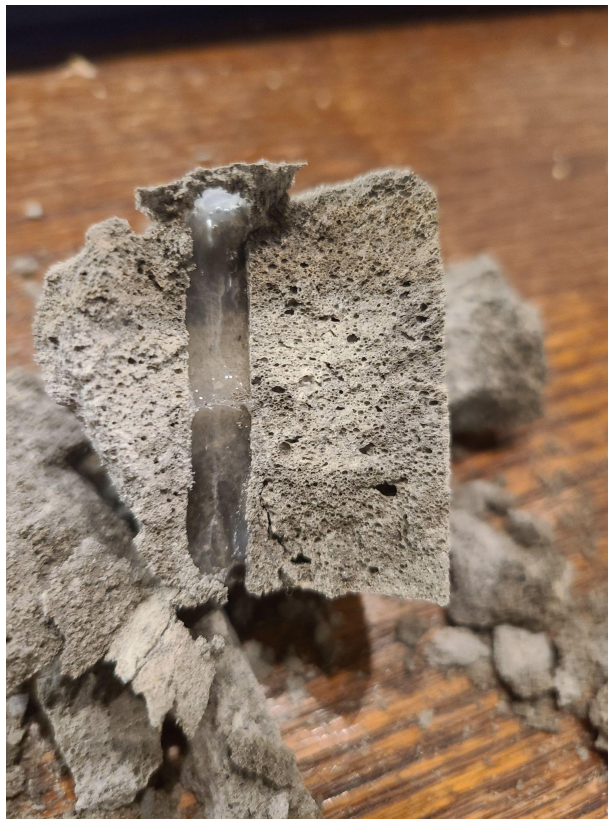
Fig 3: CO2 Sequestered Sample Cross Section
