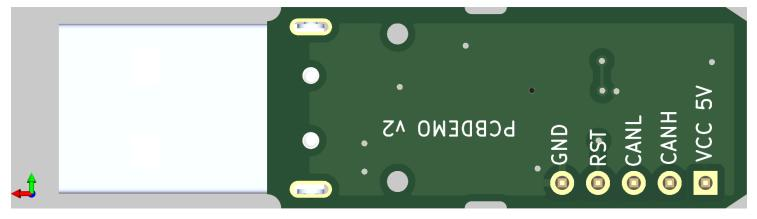
The makefile will crop the images to the PCB outline. To allow for this to happen, goto the 3D veiewer preferences and set the color gradient start and stop color to the same RGB value, here I used (200,200,200). The crop will not pass the 3D axis symbol, so place the PCB image close to this symbol.
