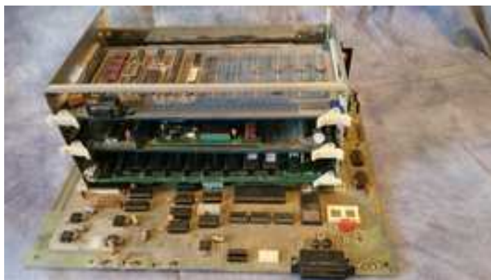
My Explorer 85 S100 Boards, Top Down: Bus Monitor+Printer Port, Magnetic Bubble Memory 32K Static RAM
