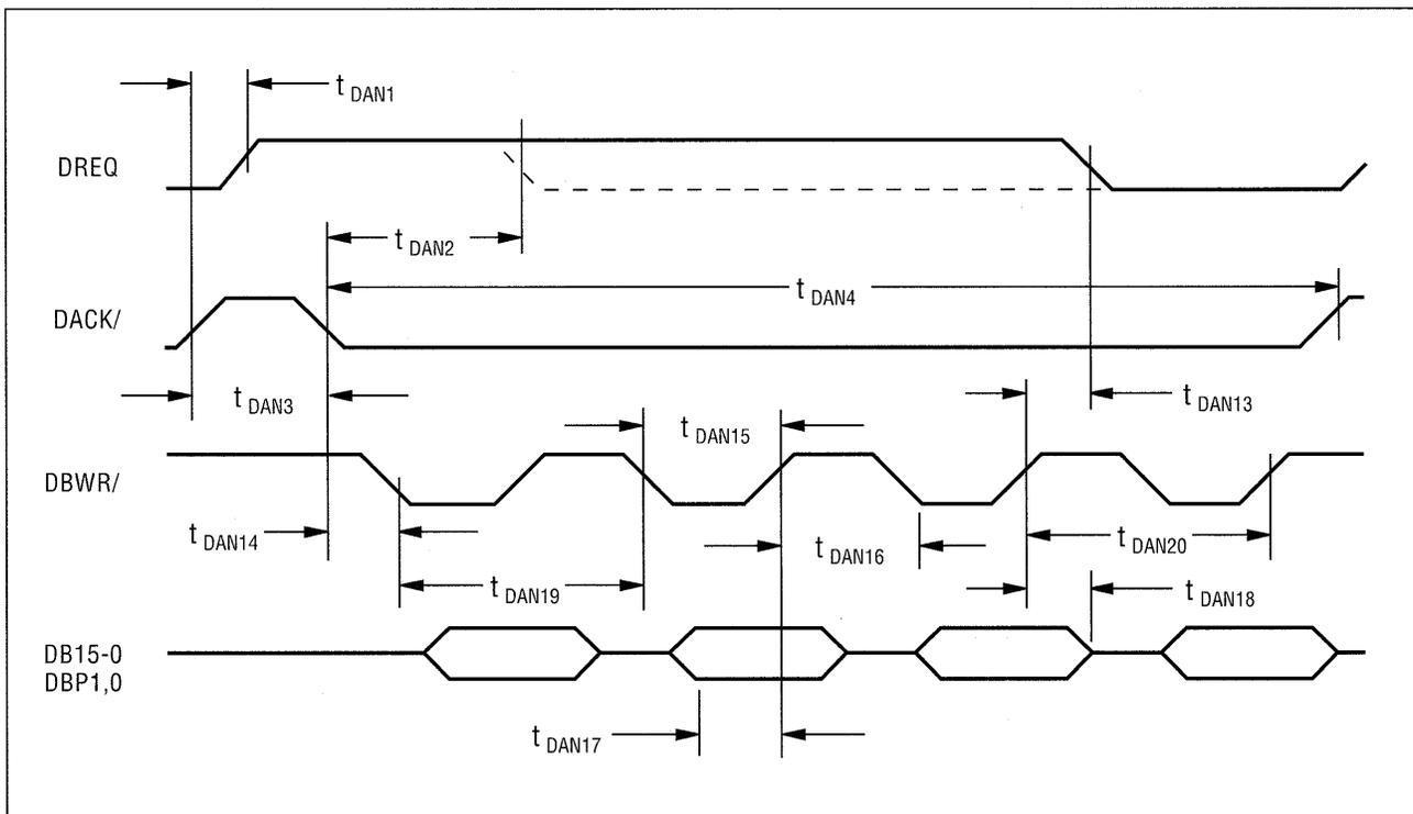
**Burst Mode DMA Interface, Nonbyte Control**
