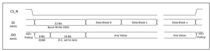
Figure 25 Burst mode write sequence
