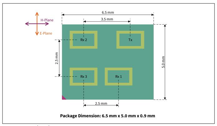
Figure 31 Top view of BGT60TR13C
