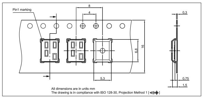
Figure 34 Tape of PG-VF2BGA-40-1
