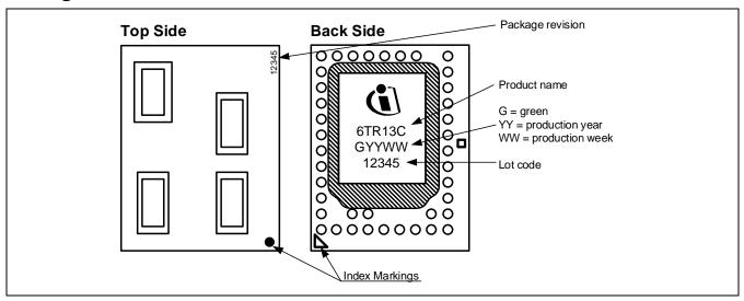
Figure 35 Marking layout of PG-VF2BGA-40-1 (example)
