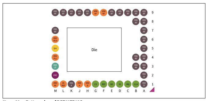
Figure 32 Bottom view of BGT60TR13C
