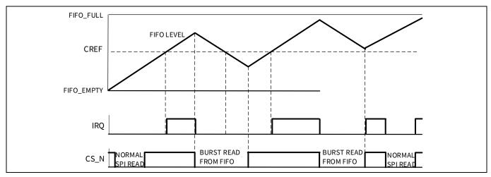
Figure 30 IRQ status behavior during radar mode with FSM capturing data
