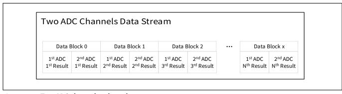
Figure 27 Two ADC channels selected
