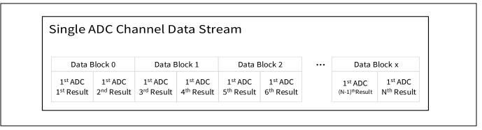
Figure 26 Single ADC channel selected
