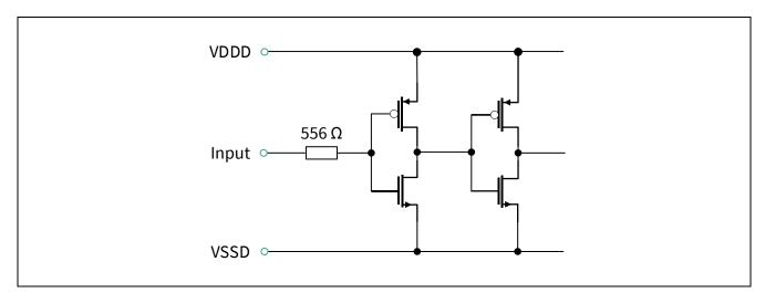
Figure 19 Interface for input pins CLK, CS\_N, DI, DIO3
