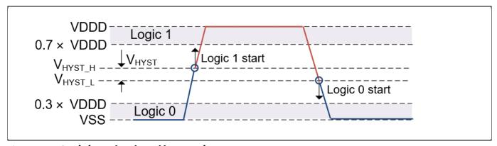
Figure 17 Logic input levels and hysteresis
