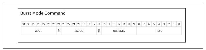
Figure 23 Burst mode command
