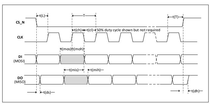
Figure 14 SPI interface timing diagram for SFCTL:MISO\_HS\_RD = 0<sub>b</sub>
