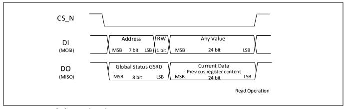
Figure 22 SPI timing read mode
