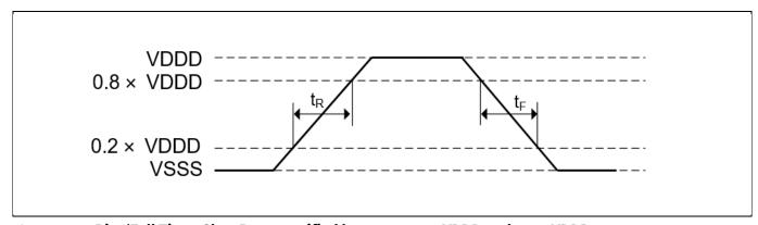
Figure 18 Rise/Fall Time, Slew Rate specified between 0.2 × VDDD and 0.8 × VDDD
