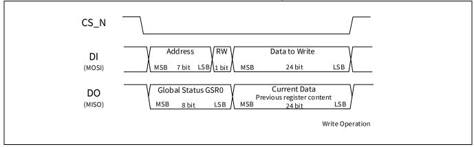
Figure 21 SPI timing write mode
