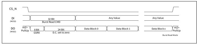
Figure 24 Burst mode read sequence
