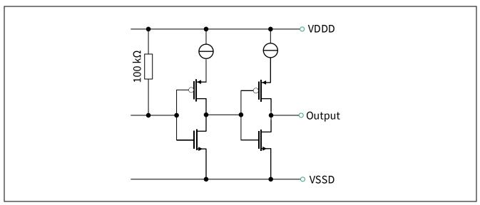
Figure 20 Interface for output pins IRQ, DO, DIO3
