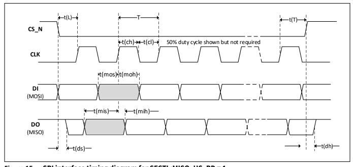
Figure 15 SPI interface timing diagram for SFCTL:MISO\_HS\_RD = 1<sub>b</sub>
