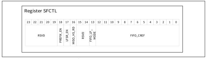
Figure 7 SPI and FIFO Control Register
