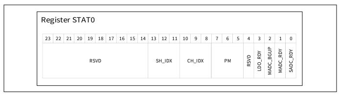
Figure 8 STAT0: Control FSM Status Register
