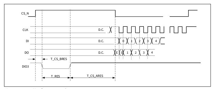
Figure 29 Hardware reset Sequence
