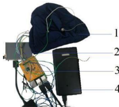
Fig.1 General View of assembled device: 1 – hat EEG, 2 – monitor, 3 – RaspberryPi and shield EEG, 4 – power bank
