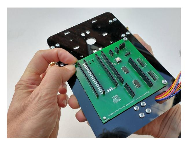
Now we can add the Trundlebot PCB we assembled before. Simply place over the screws in the orientation photographed. Screw on the remaining nuts and tighten fingertight. Connect the left stepper motor (the side of the connectors) to "Stepper Motor 1" and the right motor to "Stepper Motor 2". The red wire should be to the bottom / front of the board.
