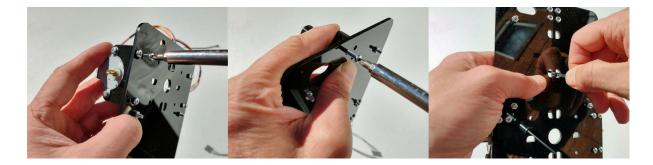
Now we need to attach everything to the chassis. First place a 10mm screw through a hole on the chassis for the PCB. You can hold the PCB over the chassis to confirm you have the right holes. Screw on a nut and tighten with your fingers, and then repeat for the other 3 holes. The side with the nut on is now the top of the Trundlebot.
