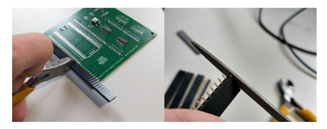
There are a couple of tricks you can use to make soldering the connectors easier. First is to use some header pins to hold the Pi Pico header sockets in place. Having some blue/Blu/white tack to hold the headers in place will also make things easier for the other connectors.
