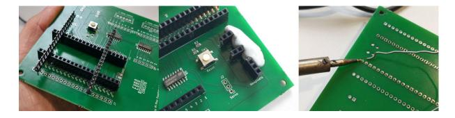
Finally when soldering long strips of headers it is good practice to solder the pins at either end, check they are straight, and solder all the pins in between.
