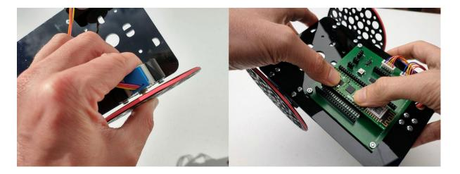
We are almost done. Now slowly but firmly push on the wheels until they will not push on any further. Now it is safe to insert your WizFi360-EVB-Pico with the USB connector facing the top/back. Finally if you have the optional battery holder printed out you can slot it in place now. The rear screws will hold it in place.
