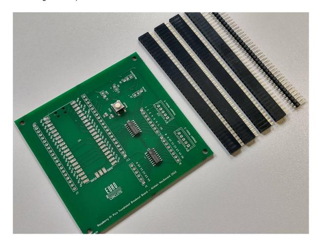
You will need the Trundlebot PCB, four 40-pin 2.54 mm pitch header socket strips, and a 40-pin 2.54 mm pitch header pin strip.
