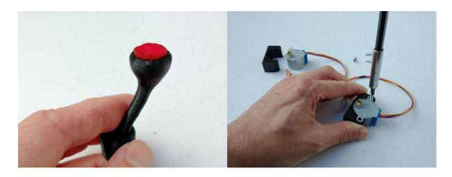
Next we need to attach the motors to the motor mounts. Simply place in the slot with the wires pointing away from the flat surface and screw in the shorter 10mm screws. The motor should not move, but be careful not to over tighten.
