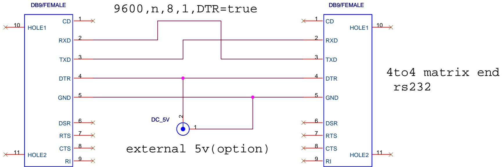
every byte of pc sending must has delaying 50ms
