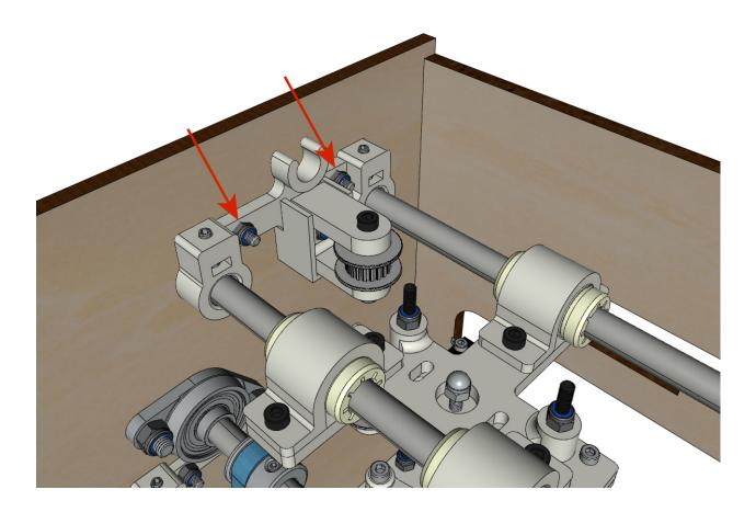
• Screw the grub screws of the axle supports on the left and right.
