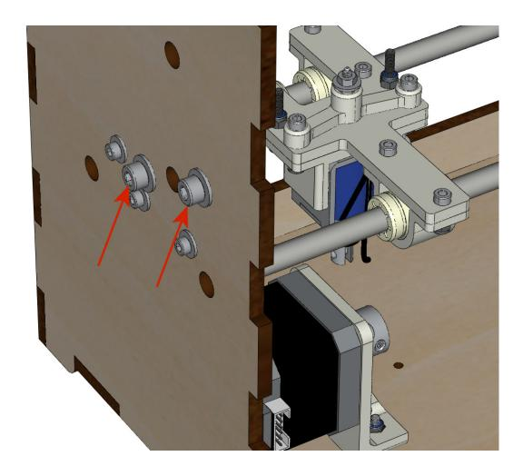
• Fix the KFL8 right on the body with the KFL8\_support, 2 screws M5-18, 2 washers M5 and the 2 nuts M5 NYL.
