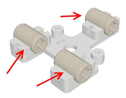
• attach the IGUS bearings with fixing collars
