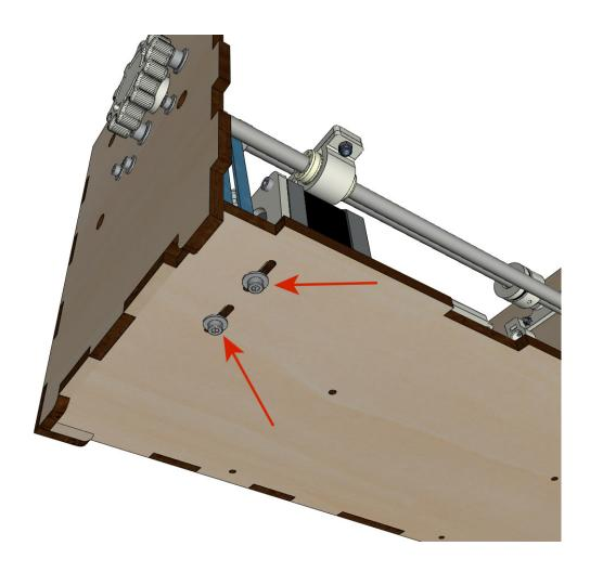
• Tighten the 2 screws of the pulley of the axle.
