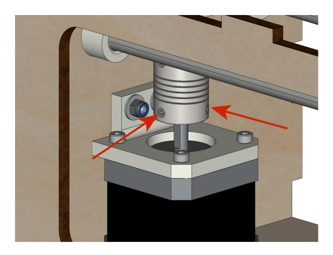
• Thread the 100mm axle into the KP08, the pulleys (respecting their positions) and the coupler.
