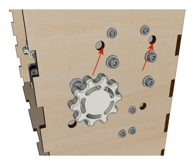
• Tighten the axle holder screws on the body on the left and right.
