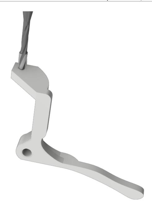
$\bullet \ \ Position \ the \ lever \ \ ENDSTOP\_Y\_LEVER \ in \ the \ support**ENDSTOP\_Y\_support**.$
