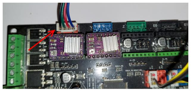
• The Y motor (paper) must be plugged into the right connector (blue)
