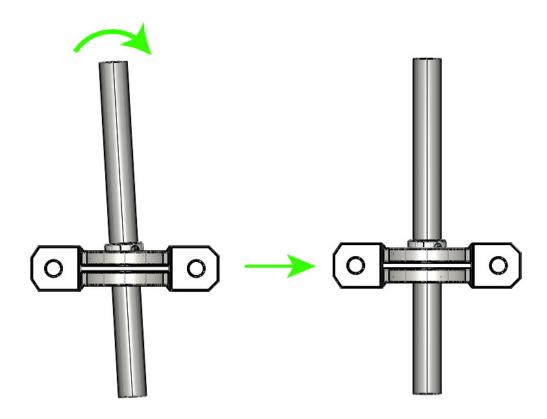
• Screw the KP08\_support and the KP08 on the body a bit with the M5-25 screws, M5 washers and M5 NYL nuts.
