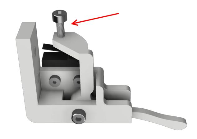
• Assemble the limit switch assembly and the SWITCH\_Y\_support to the body using the M3-14 screws, M3 washers and M3 NYL nuts.
