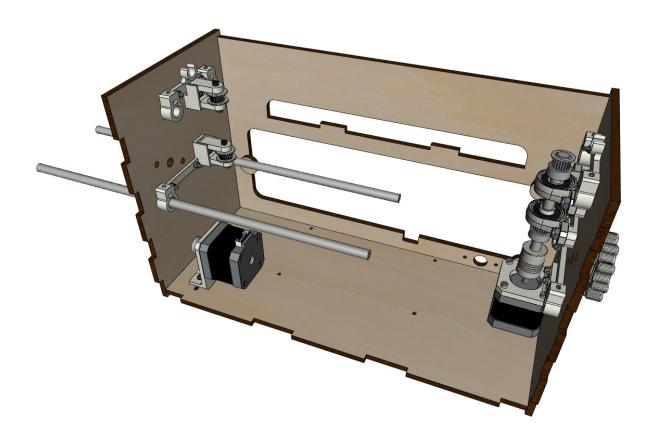
$\bullet\,$  Thread the switch and its support on the Ø8mm bar on the back side.
