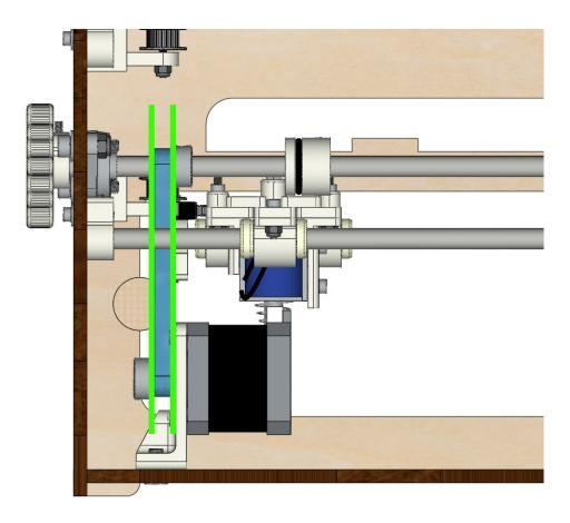
$\bullet$  Move the Y motor / support assembly along the oblong holes under the body to tension the closed belt and tighten the 2 screws.
