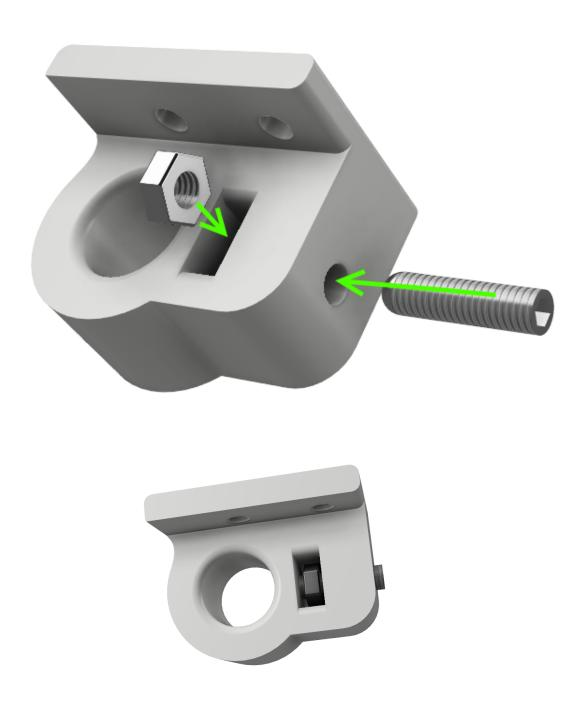
• Screw the limit switch to its support (SWITCH\_X\_support) using M2.5-14 screws and M2.5 nuts.
