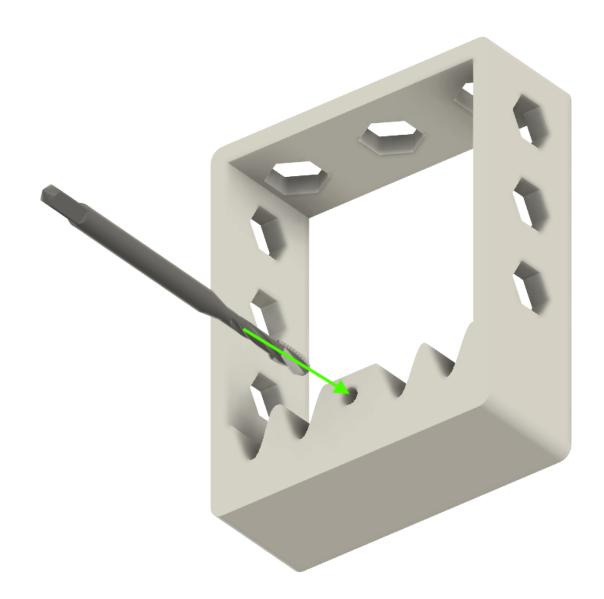
• Fix the two parts printed **YMOTOR\_support2\_200\_2** and **YMOTOR\_support2\_200\_1** with an M3-12 screws.
