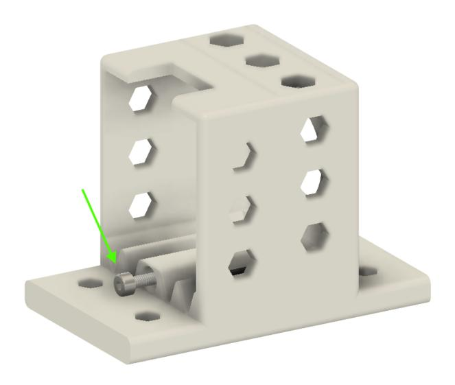
• Fix the part **YMOTOR\_support2\_200** on the previous set with a M3-12 screws.
