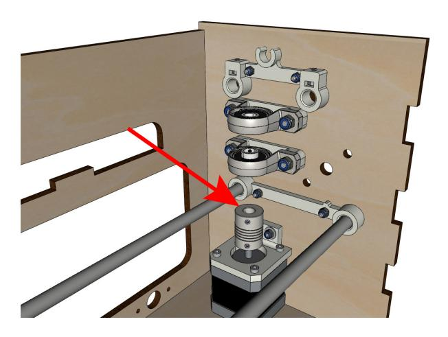
• Thread the 100mm linear shaft from the top through the KP08 and into the coupler.
