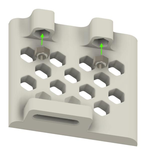
• Fix the two parts printed **XMOTOR\_support2\_1** and **XMOTOR\_support2** with two M3-14 screws.
