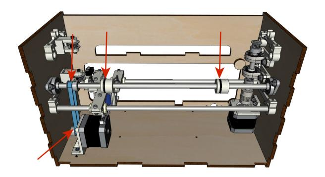
$\bullet$  Press the axle into the right KFL8 and cross it so that it protrudes  $\pm$  12mm from the body.
