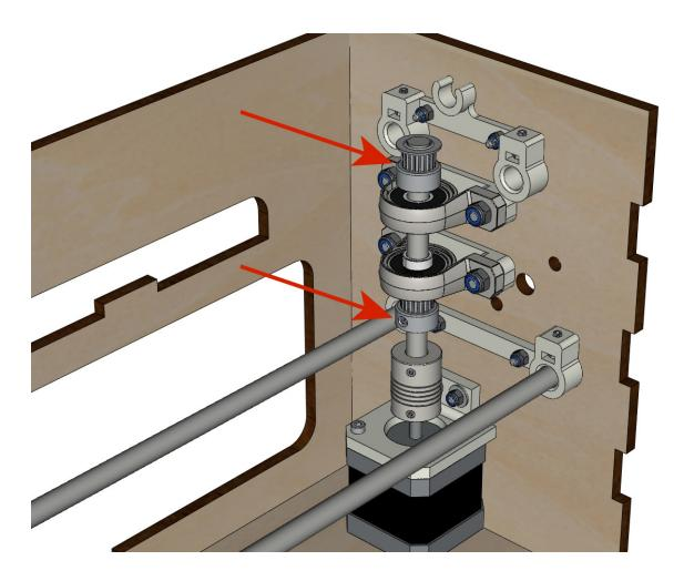
• Screw the 2 screws at the top of the coupler onto the vertical axis.
