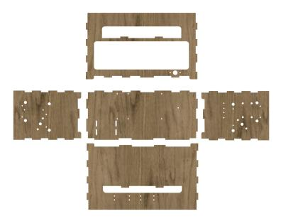
• Glue the notches, assemble the 5 parts and hold them in place with painter's tape the drying time recommended by the manufacturer.
