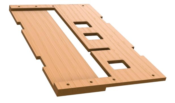
**Attention:** the 2 parts must be perfectly aligned. Place screws in drillings to properly align the parts. There must not be any of space between the two pieces (where the sheet of paper could come jam). Tighten the parts well against each other with clamps
