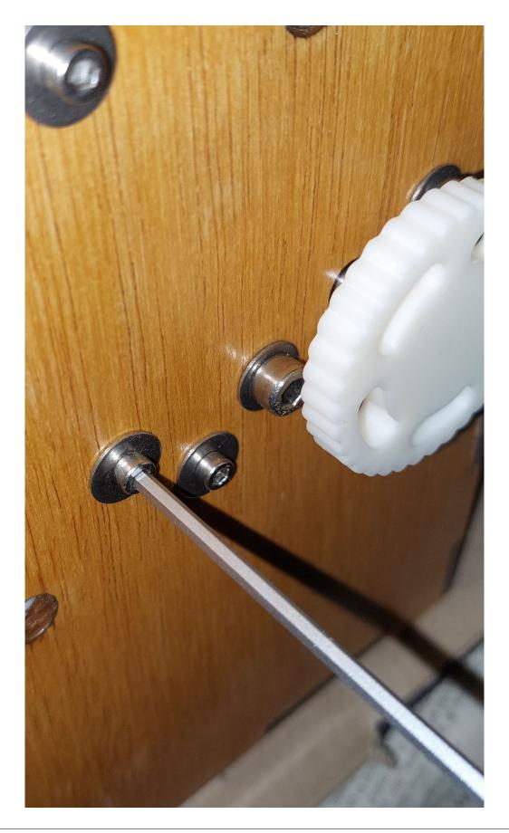
**Note:** For now, do not tighten the pulley bolts on the axle.
