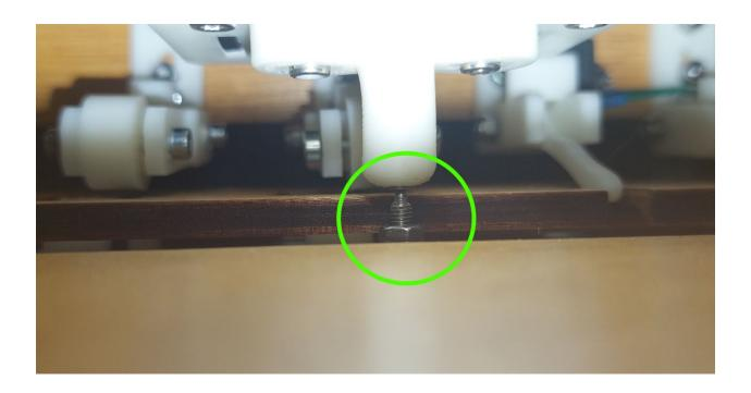
• When the alignment is satisfactory, lock the upper pulley onto the vertical axis.
