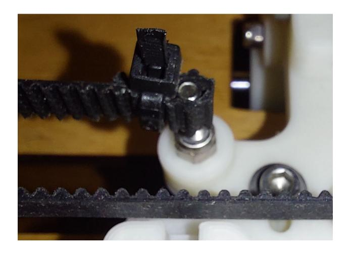
• Pass the belt in the free pulley then the pulley of the vertical axis.
