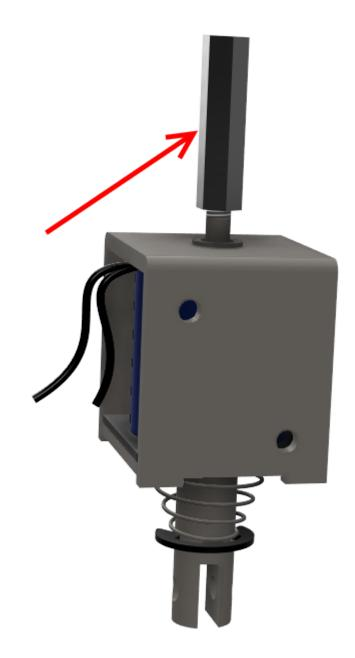
• Tighten the M3-12 screw with the Braille stylus punched out, allowing it to extend  $\pm$  6mm beyond the spacer.
