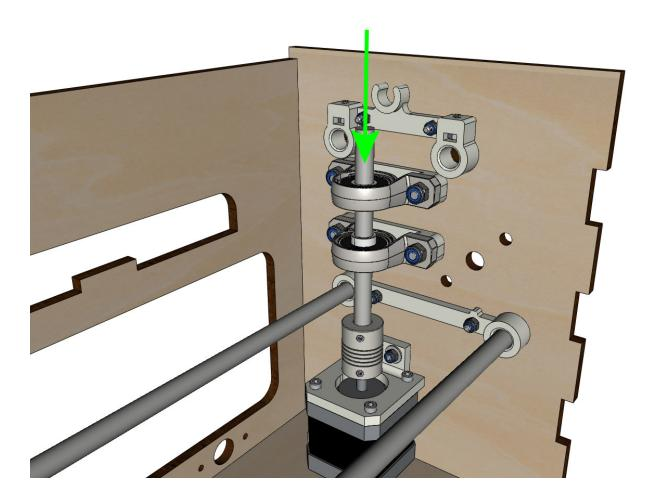
• Rotate the linear shaft by hand to ensure that all elements are aligned and that the spindle continues to rotate freely.
