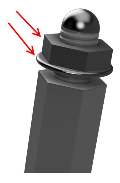
**Note:** The axis of the electromagnet must be able to move up and down freely without resistance.
