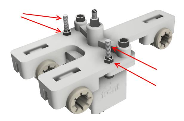
• Fit a washer and tighten the M3 lock nut, ensuring that the stylus screw does not move into the spacer at the same time. The washer prevents the jam nut from getting caught in the spacer guide.
