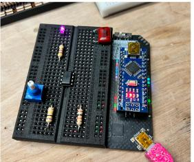
The breadboard has 144 through hole soldering joints and the top has 33
