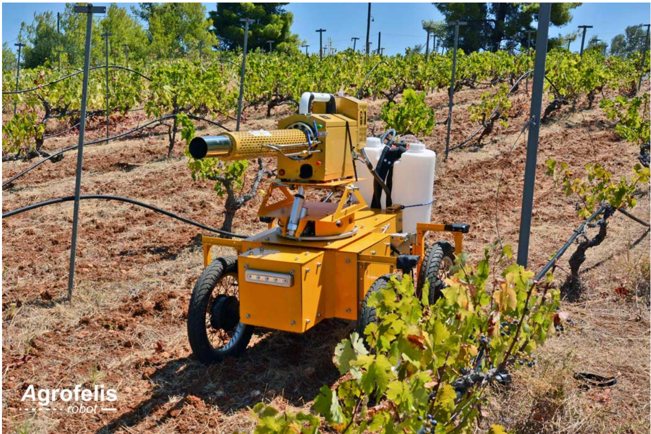
Figure 3: Agrofelis Robot in the vineyard downhill with a pulse jet fogger
