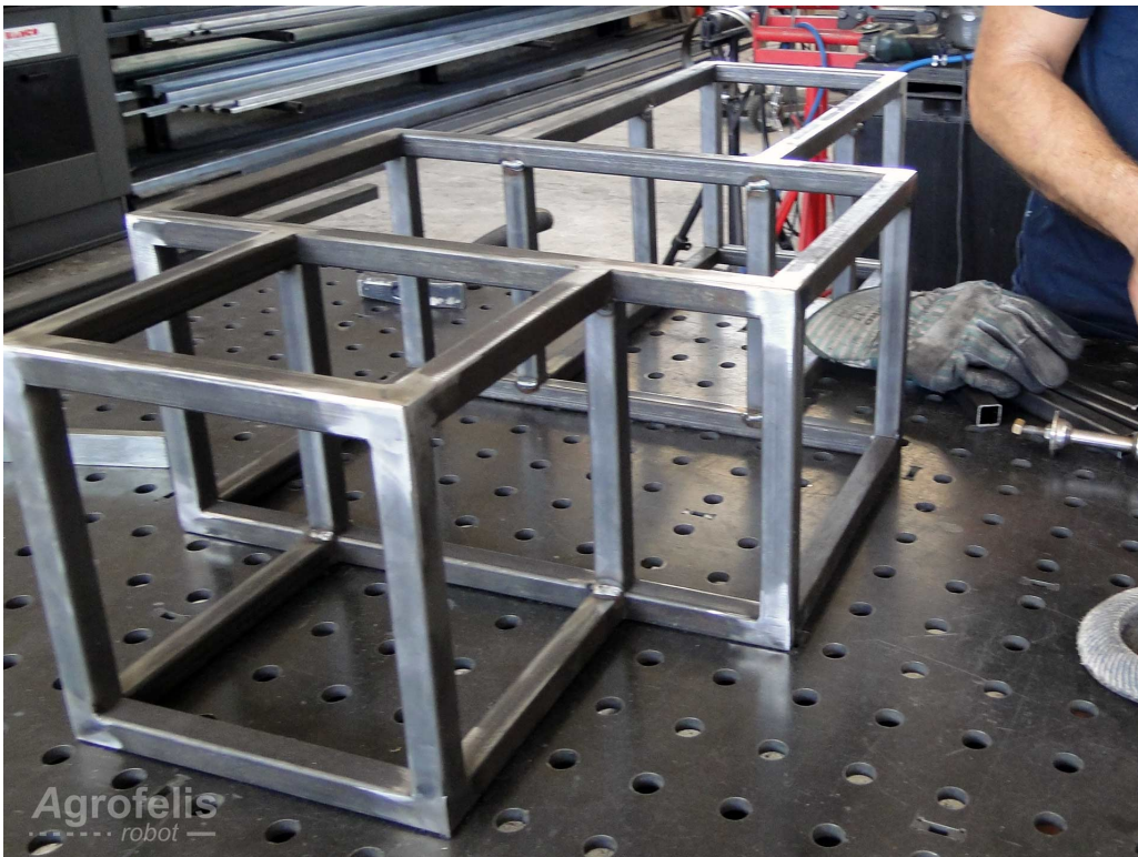
Figure 11: Manufacturing the frame step 4, fabricating the middle bars, completed
