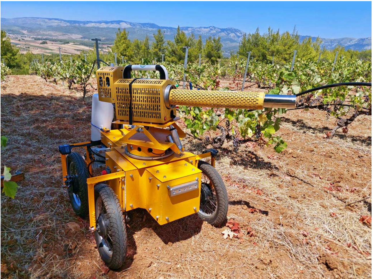
Figure 1: Agrofelis Robot in the vineyard with a pulse jet fogger
