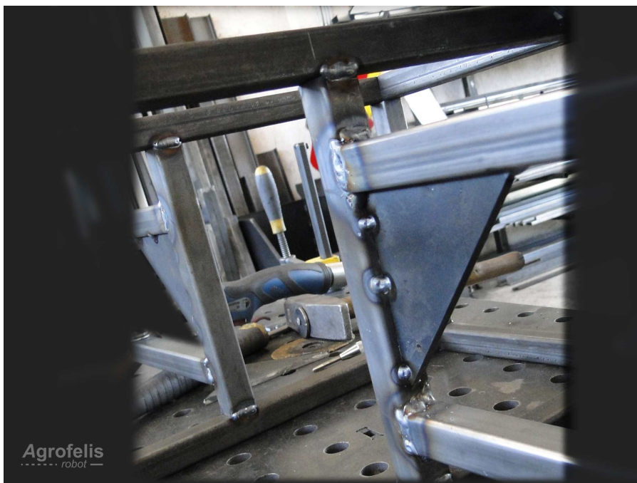
Figure 13: Manufacturing the frame step 5, back wheels attachment fabricated
