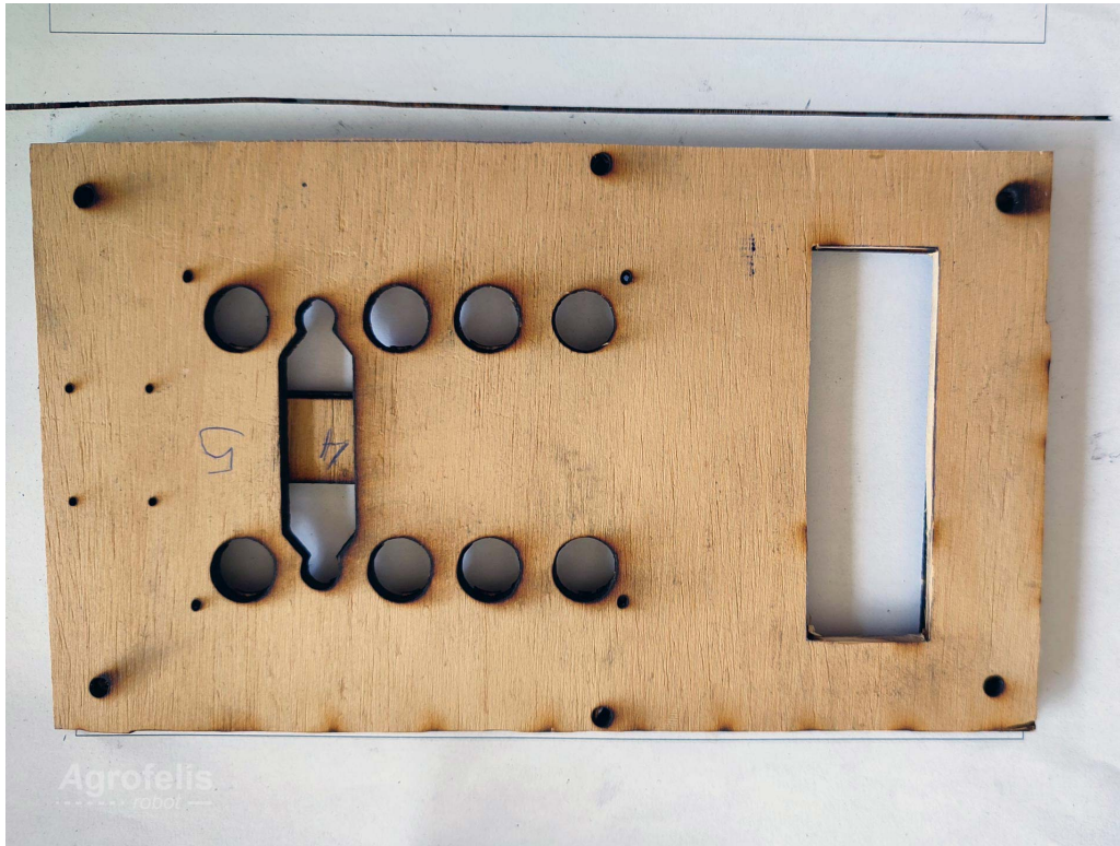
Figure 6: Two laser cut layers of 4 mm plywood stacked to form the top body of they structural element.
