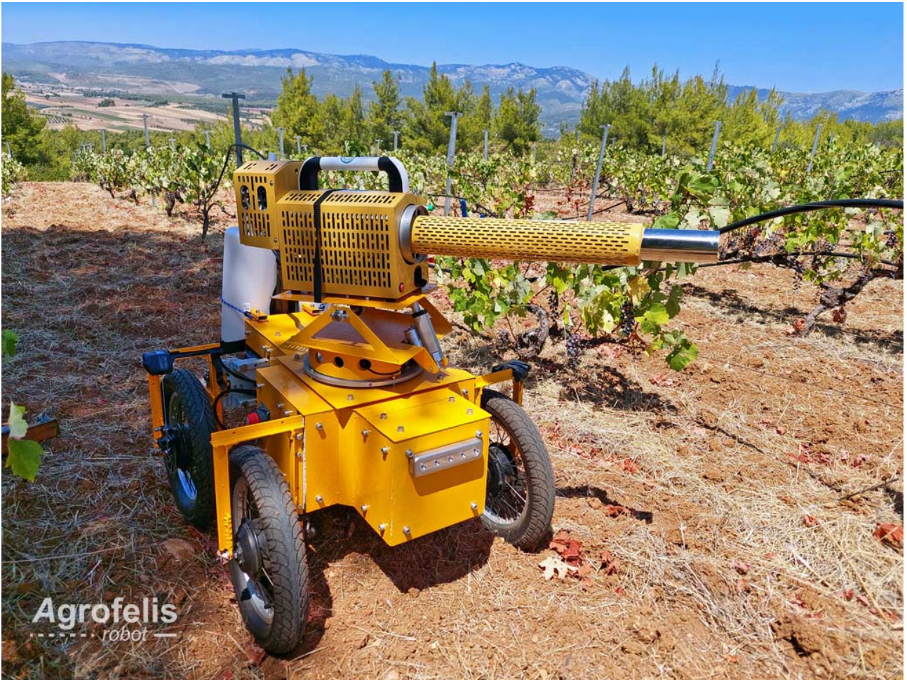
Figure 28: Agrofelis with the implement mount in a vineyard
