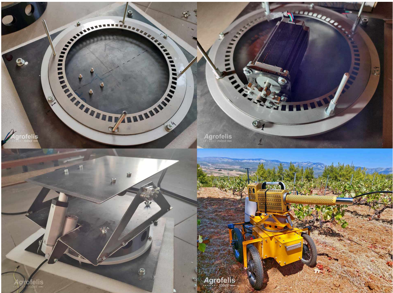
Figure 12: Agrofelis two degrees of freedom rotating implement mount figures highlights
