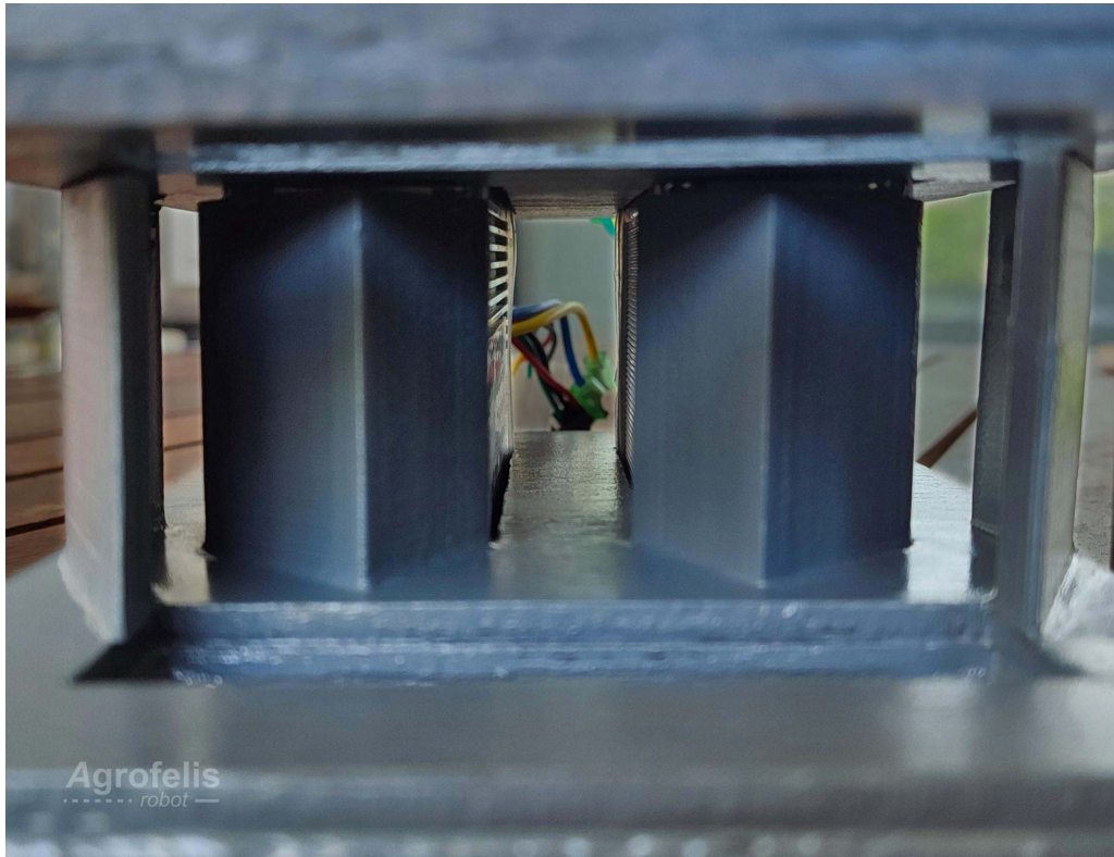
Figure 8: A front view focusing on the 3d printed air fins guiding the airflow on both sides of the motor drivers
