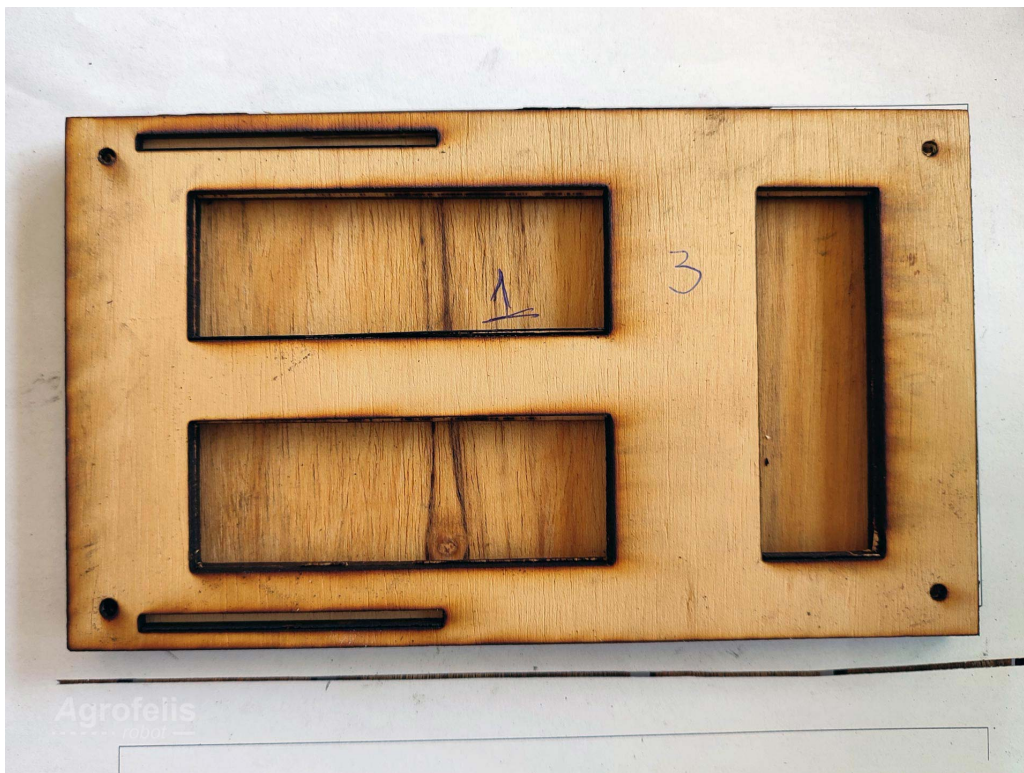
Figure 5: Three laser cut layers of 4 mm plywood stacked to form the bottom body of structural element
