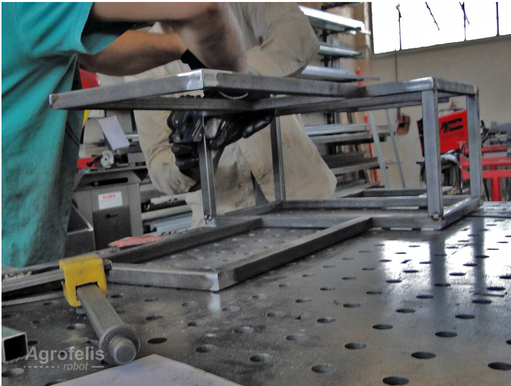
Figure 10: Manufacturing the frame step 4, fabricating the middle bars in progress
