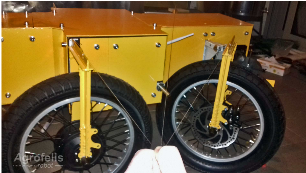
Figure 30: Ackerman and wheels manual adjustment
