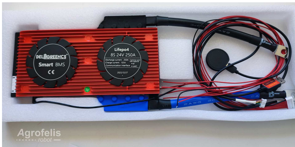
Figure 11: BMS with peripherals
