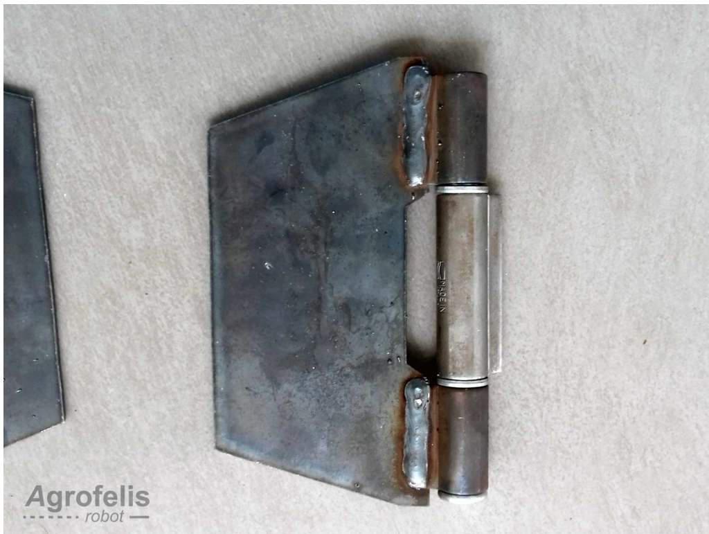
Figure 14: Hinge mount fabricated view a
