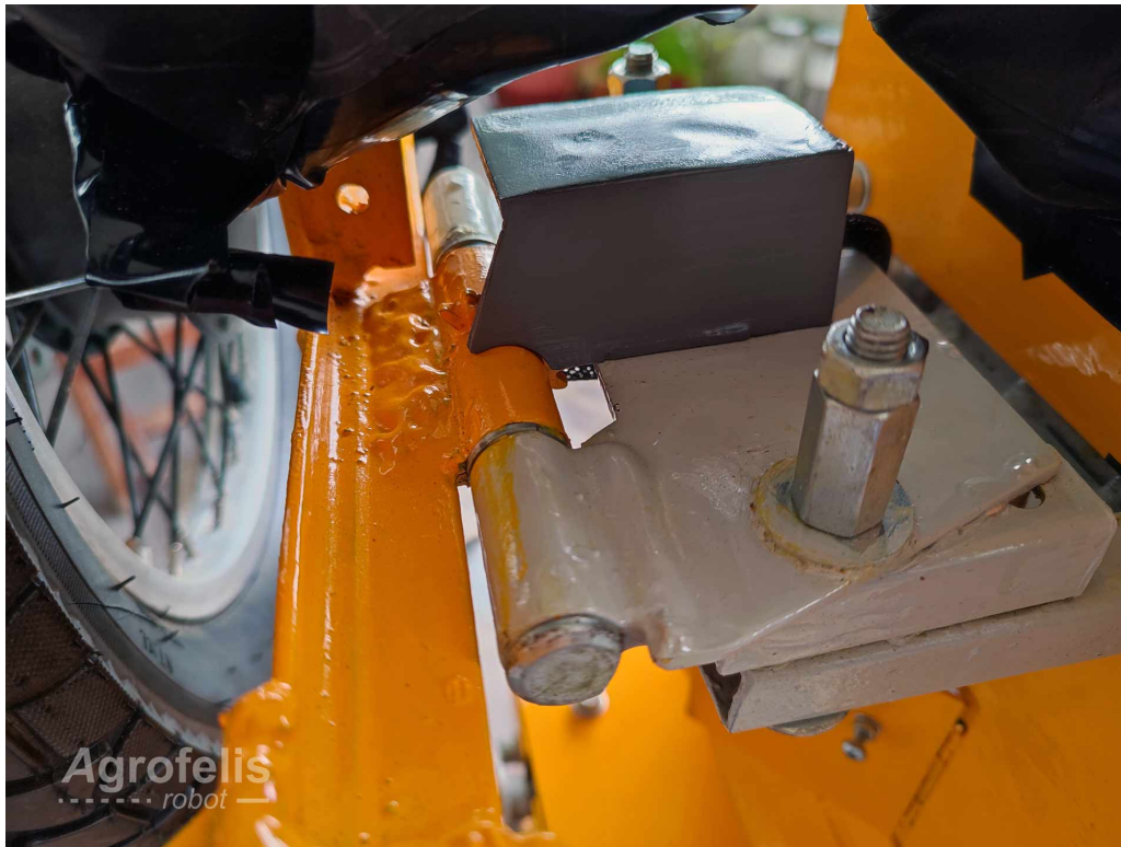
Figure 17: Hinge mount fabricated view d
