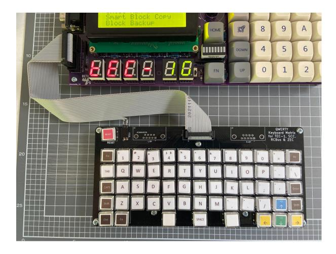
To activate the Keyboard, The Matrix switch on the 3-DIP switch is to be turned on. This activates the Matrix Keyboard and disables the onboard Hex Keypad (except Reset). Mon3 only maps keys present on the TEC-IG to the Matrix Keyboard.
