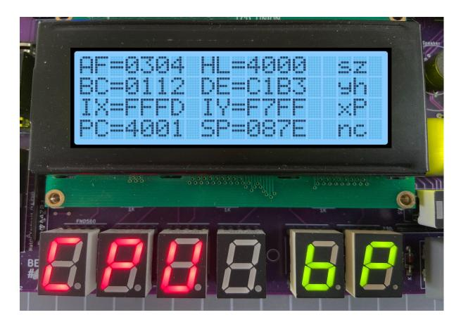
The contents of the Z80 CPU registers AF, HL, BC, DE, IX, IY, the Program Counter and Stack Pointer are displayed. CPU Flags are also displayed. Flags that are set are in Capitals. To continue code execution press the GO key and to quit execution and return to the Monitor press the AD key. Finally, to remove an inserted Breakpoint press Fn-Minus at the address where the Breakpoint is. This will remove the breakpoint and adjust the code to its original state.
