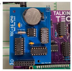
To initially set the RTC, a convenient RTC Setup routine has been provided in the Settings item in the Main Menu. Select "**Configure RTC**". Press the following keys to update the time/date: 0 = Hour, 1 = Minute, 2 = Second, 3 = 12/24h, 4 = Day of week, 5 = Day, 6 = Month, 7 = Year, 8 = View RTC PRAM, F = Reset RTC, AD = Exit. When viewing RTC PRAM data, Plus = Move Down, Minus = Move Up, AD = Exit back to RTC Setup.
