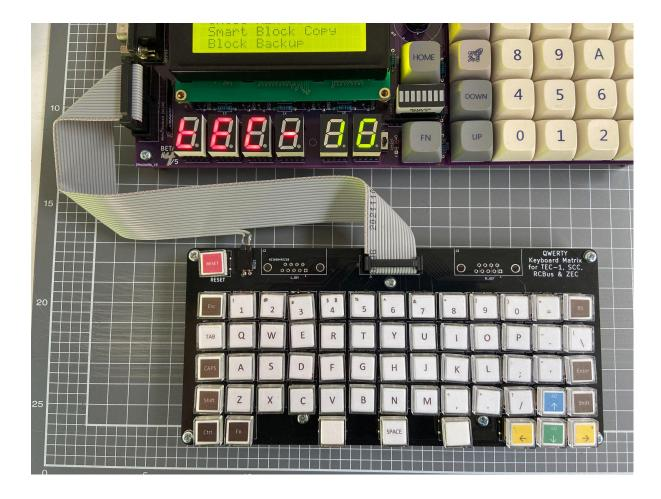
To activate the Keyboard, The Matrix switch on the 3-DIP switch is to be turned on. This activates the Matrix Keyboard and disables the onboard Hex Keypad (except Reset). Mon3 only maps keys present on the TEC-1G to the Matrix Keyboard.
