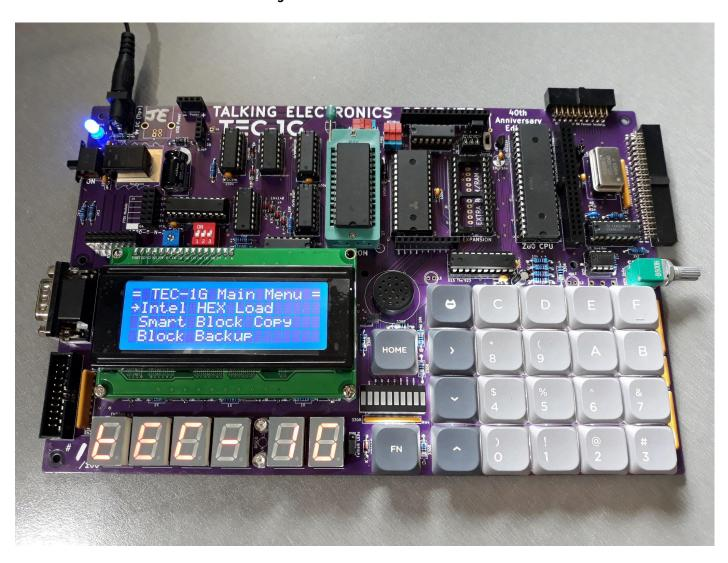
Mon3 (Talking Electronics Computer Monitor version 3) is custom-built for the TEC-IG Single Board Z80 Computer. Mon3 is the heart of the TEC-IG. It brings the hardware to life. Consider it an Operating System that provides the ability to program the TEC. The monitor is jam-packed with features, designed for beginners who are just learning to code Z80 and rich enough for the advanced software developer.
