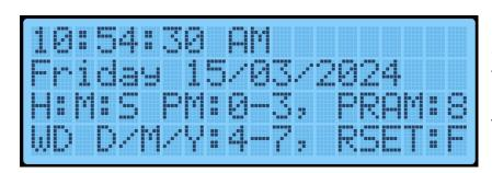
Mon3 will automatically utilise the internal PRAM to retain some settings when the TEC-1G is powered down. 14 Free bytes are
