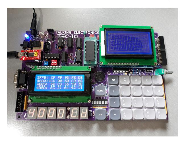
The GLCD library contains a variety of routines that can produce simple shapes and lines, these include text, lines, rectangles, circles and pixels.
