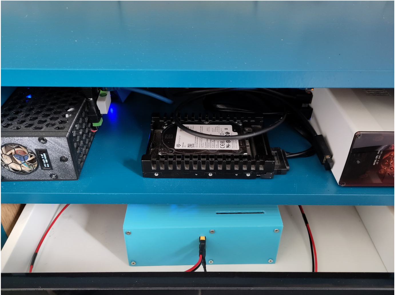
Fig.1. The UPS powers two small board computer based servers: a NAS and a Nextcloud/Homeassistant server.
