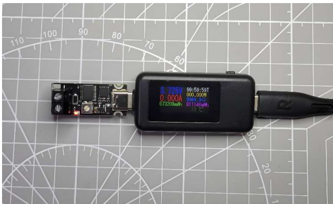
Voltage can be adjusted from 3.3V to 21V
