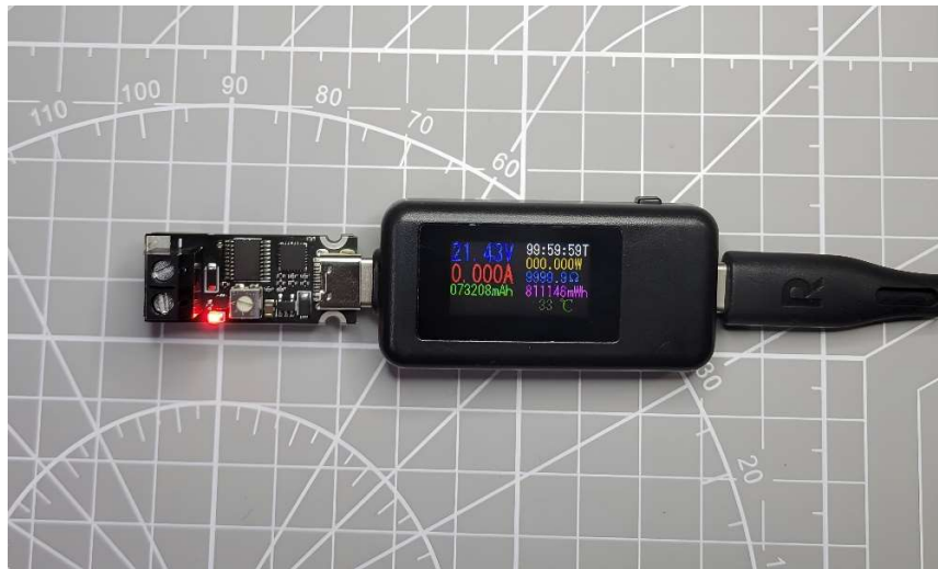
Set max voltage at 21V at no load.
