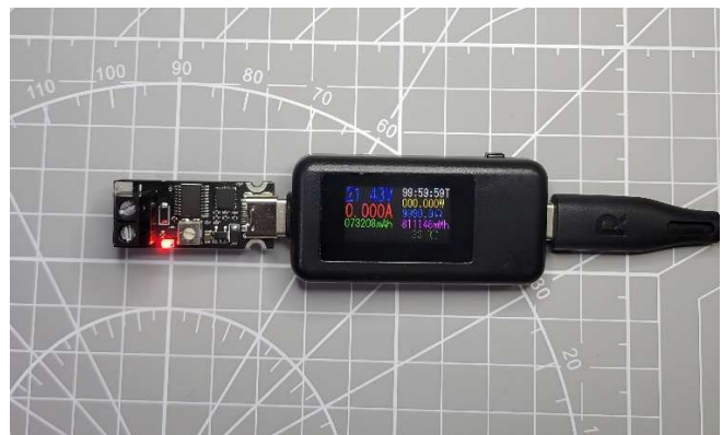
Voltage can be adjusted from 3.3V to 21V
