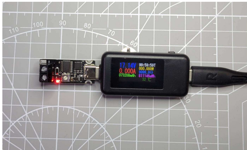
Set max voltage at 17.1V at no load.
