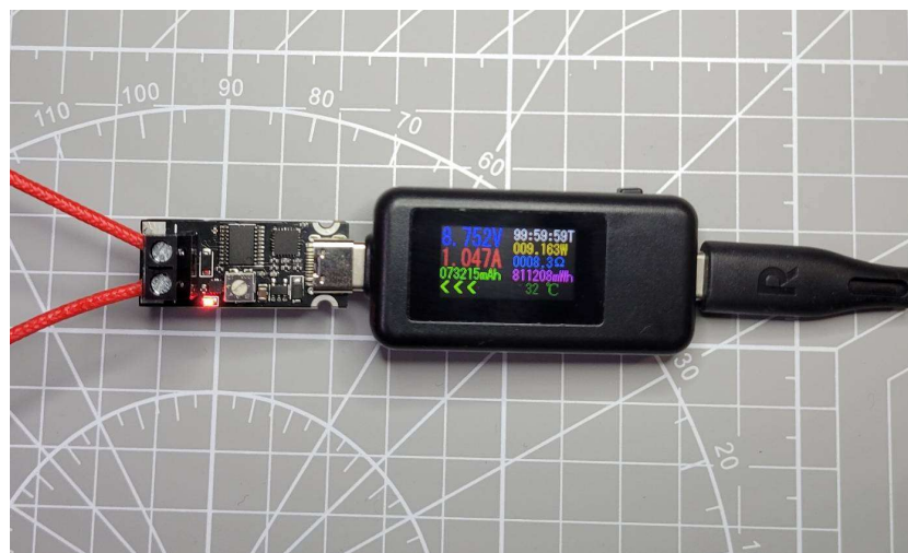
Attaching 8 Ohm load reduce voltage to 8.75V to maintain 1A current limit.
