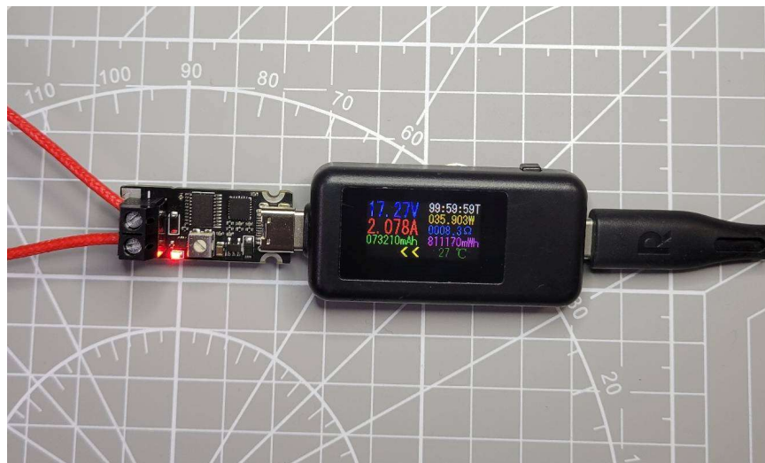
Attaching 8 Ohm load reduce voltage to 17.3V to maintain 2A current limit.
