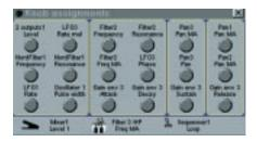
The "knob floater" is a useful tool on the monitor screen to display your knob assignments.
