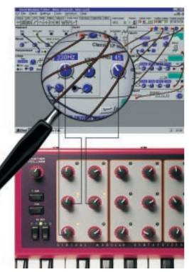
All parameters in the patch are assignable to knobs on the Modular. Highlight the parameter of your choice and assign it to a knob. In this example, the parameters Filter frequency, resonance and envelope amount are assigned to the three marked buttons on the Modular.
