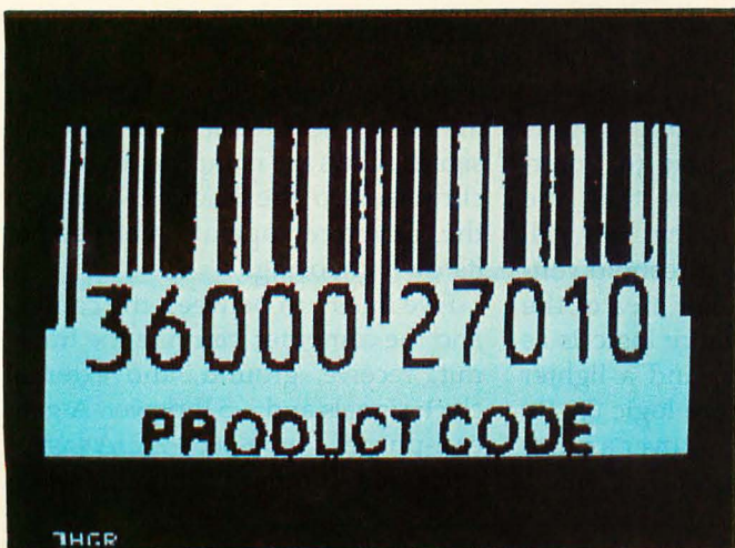
Photo 2a: The Micro D-Cam can focus on UPC bars. Both photos shown here used the Apple II's high-resolution graphics routines to reproduce the camera's output.
