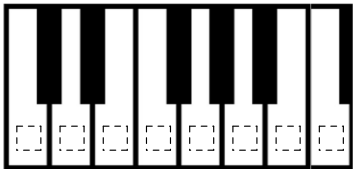
Do Re Mi Fa So Ra Si Do Touch pad made by PCB pattern and silk
