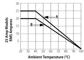
A: Single relay or with 0.75" spacing between relays. Derate above 40 °C; subtract 0.5 amp/°C.
