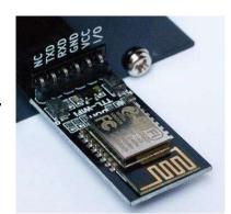
At any time, the module can be reset to factory default settings by keeping the button labelled **G** pressed until the LED turns off.
