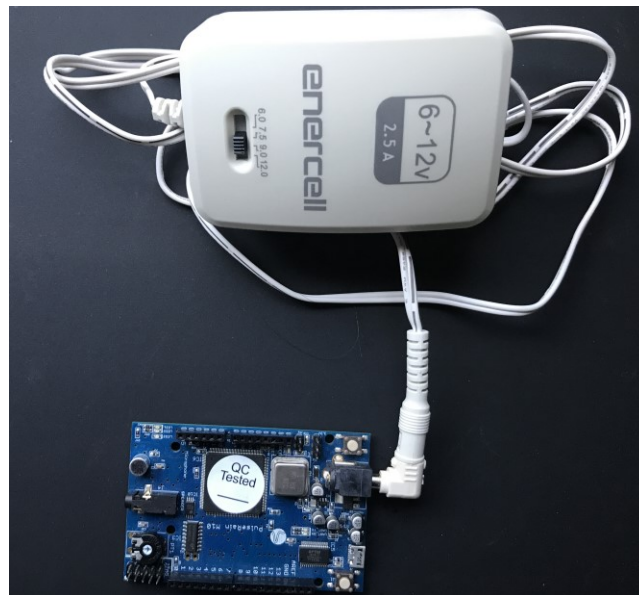
Figure 1-4 Supply Power through DC Jack (7V – 12V)
