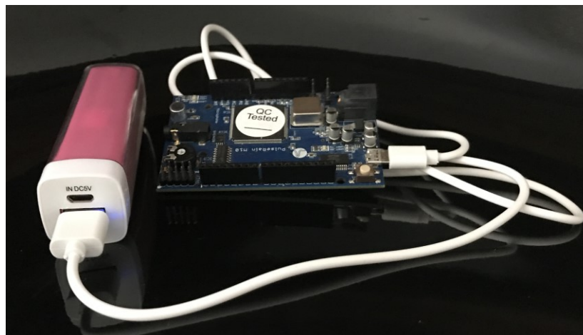
Figure 1-5 Supply Power through microUSB
