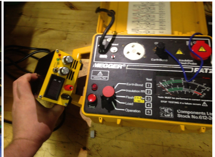
Being Used in anger! Seems to power this dismantled Tablet just fine. Gave it a PAT inspection too.
