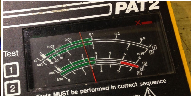
Earth bond test position 1 and the result
