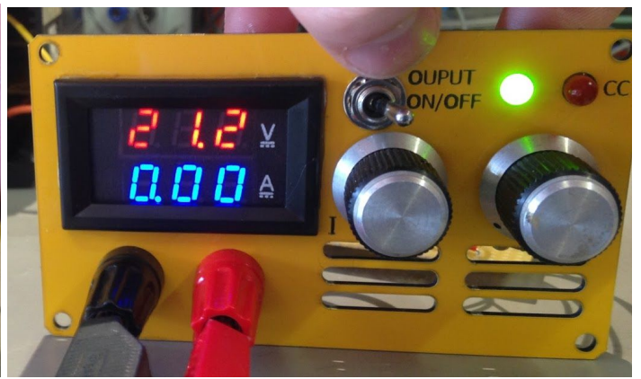
Display was tested to check voltage on output with output off.
