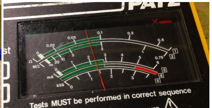
Earth Bond test position 2 and the result
