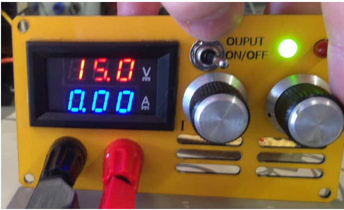
Display was tested to check voltage on output with output off.
