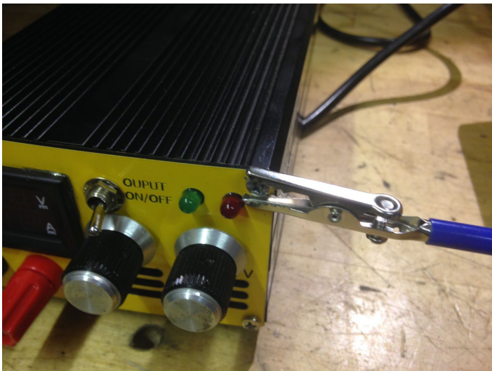
Earth Bond test position 2 and the result
