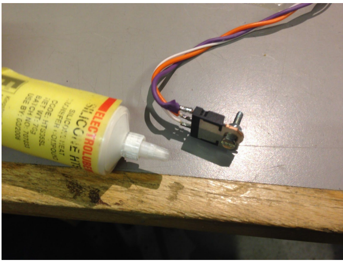
Applied a small amount of thermal paste to transistor and bolted it to slot in case roof with modified M3 bolt (sides of bolt head we're squared off)
