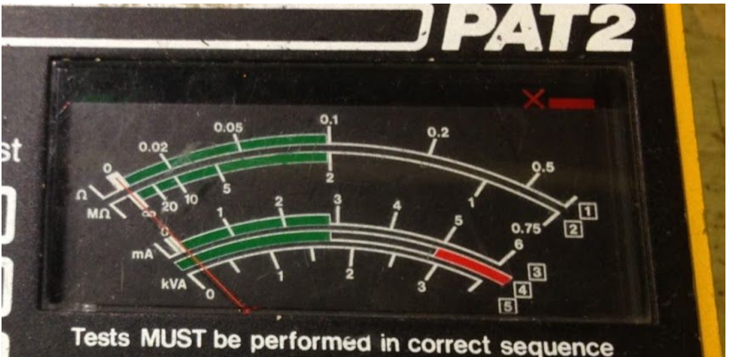
Insulation test result and Earth bond test position 2. All good! All Safe!
