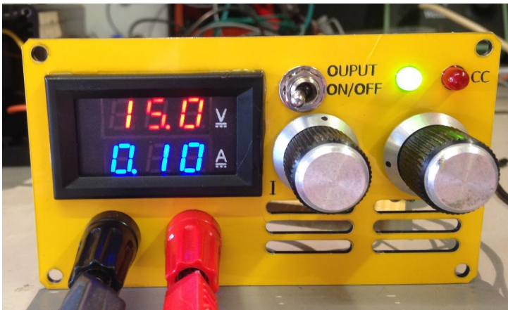
Load test at higher voltage with 150R load.
