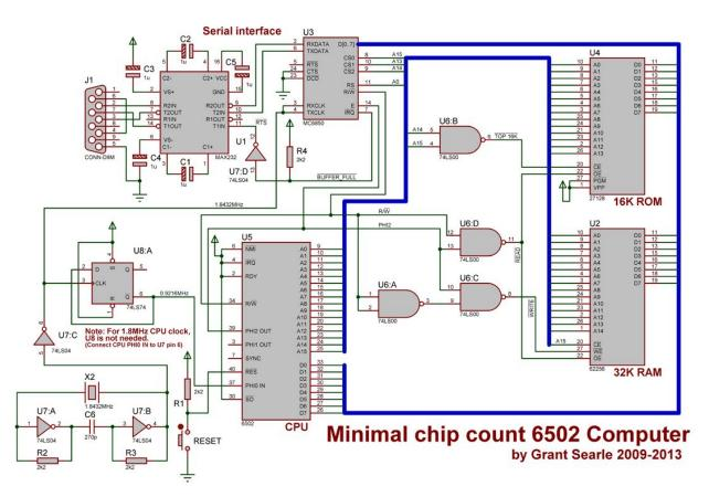
This creates the following memory map: 0000-7FFF 32K RAM 8000-9FFF FREE SPACE (8K) A000-BFFF SERIAL INTERFACE (minimally decoded) C000-FFFF 16K ROM (BASIC from C000 TO DED3, serial routines FF00 to FFFF, so a large amount of free space suitable for a monitor etc)
