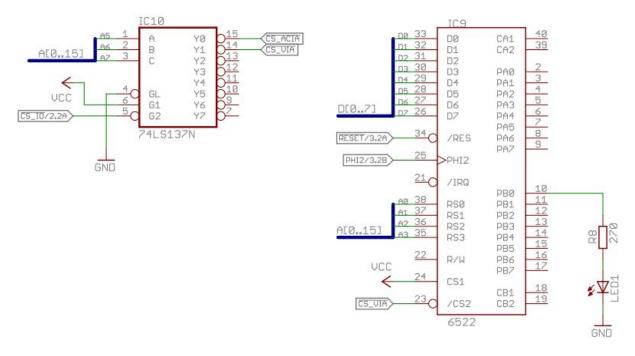
For CS2, run them to the appropriate Y connector of the SN74LS138 (Y0 to Via1 and Y1 to Via2).
