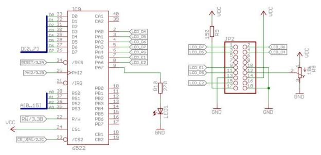
Note that in my case I didn't need to connect an E2(Enable 2) pin, since my lcd only has 2 lines, and therefore only had one enable pin. So just ignore the connection going from PA6(pin 8) of the via.
