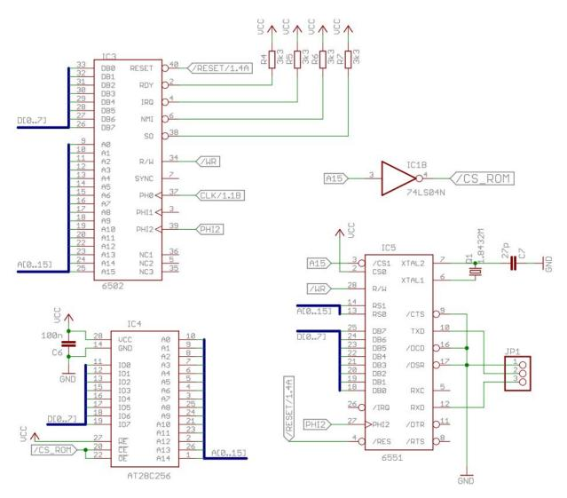
Instead of the 1.8432 crystal I used a can oscillator attached to xtl1 only. A0 is hooked to rs0, A1 is hooked to rs1. cs1 is hooked to A14, and A15 is hooked to CS0. This way when the cpu accesses A000 the binary looks like 1010 for A, A15 is high and A14 is low, thereby selecting the chip.
