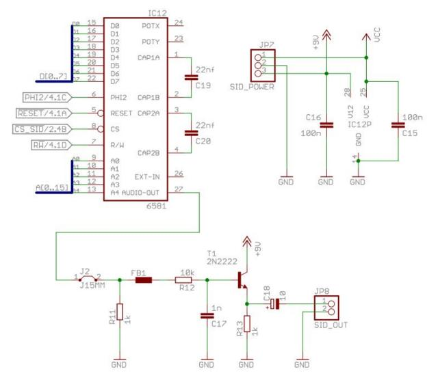
For the audio out circuitry I stuck a 1k resistor from the 6581 pin 27 to ground and then ran the signal over to an amplifier built from an Im386 circuit found here:
