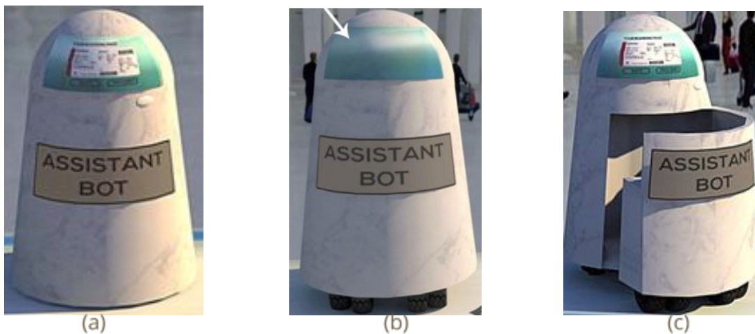
Figure: (a) Assist bot under charging condition; (b) Bot in deployed (activated) condition; (c) Change in structure of bot for allowing physically disabled people to sit
