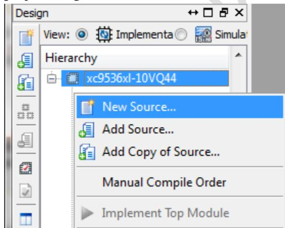
This will allow us to add the required VHDL source file as well as the User Constraints file [UCF] used to assign our pin definitions. Once the Select Source Type dialog has appeared make sure you select [VHDL Module] then give it a name like "tut1main", using main at the end allows you to quickly identify what file is the top most part of your source code.
