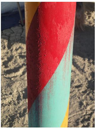
Paint Scars from Aerodynamic Heating
