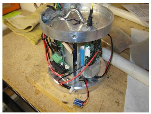
Booster Av-Bay, showing the Raven (left) and Beeline GPS (right). At the bottom is a tapered hole where a screw secures the N1000 motor to the av-bay. The GoPro camera faces out opposite the Beeline.
