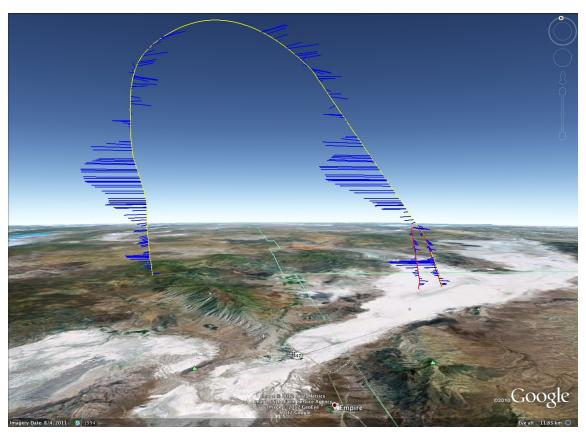
Full Flight 1 – GPS Tracking and Wind Overlay
