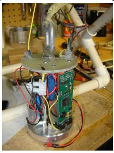
Sustainer Av-Bay, showing the Beeline GPS unit (left) and R-DAS Tiny (right). The Raven is on the far side.
