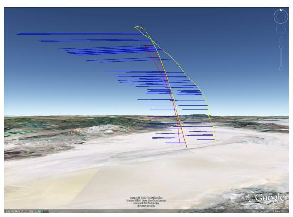
Full Flight 3 – GPS Tracking and Wind Overlay
