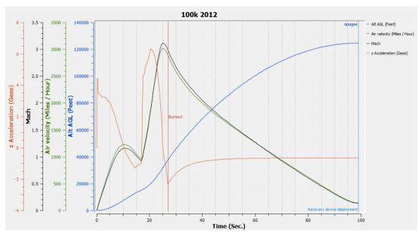
N.B., the velocity curve in the simulation graph is mislabeled; the velocity is in fps. Simulation: Ken Biba
