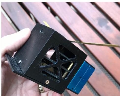
Some sensors - like the particulate matter sensor, the experimental multispectral imaging board or the radiation sensor can be packaged externally - mounted to the aft side of the package.
