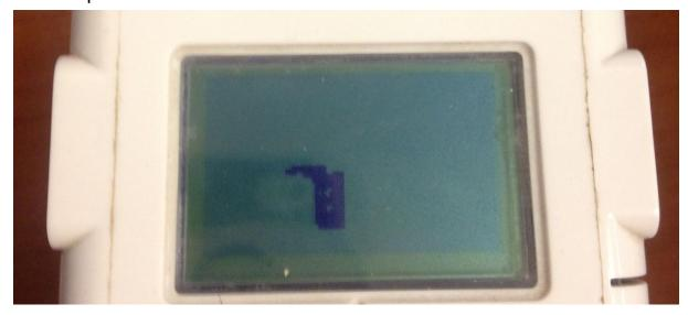
The obtained image is distorted due to stretching the width of the image with respect to its height.
