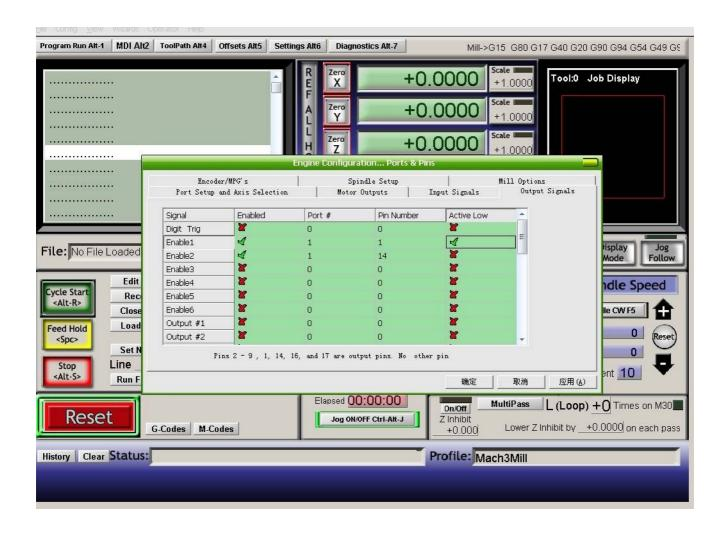
9. Spindle setup in "Ports and Pins" menu to click "Spindle Setup", set as below, and then save.
