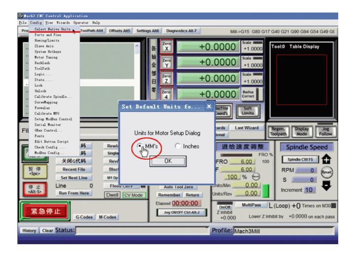
3. See as below, open "Config--Ports and Pins" to enter the setup.
