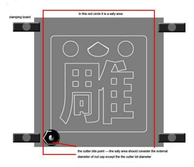
Notice:when doing holed-out work, please put a no-use flat board below the material to avoid the damage of the working station
