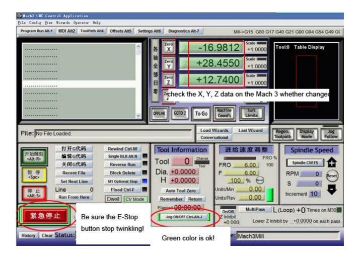
If all the axis can move, please check the direction of the axis coordinate is right(see below). If you find the axis which move wrong direction please change the setup as Page10 green letters.
