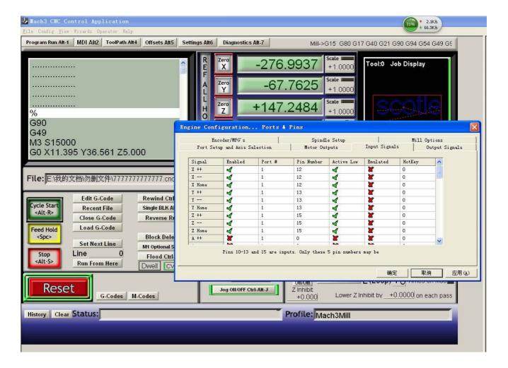
8. Output signals setting in "Ports and Pins" menu to click "Output Signals", set as below, and then save.
