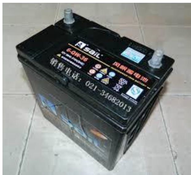
[Figure - 4.4 Lead-acid battery]
