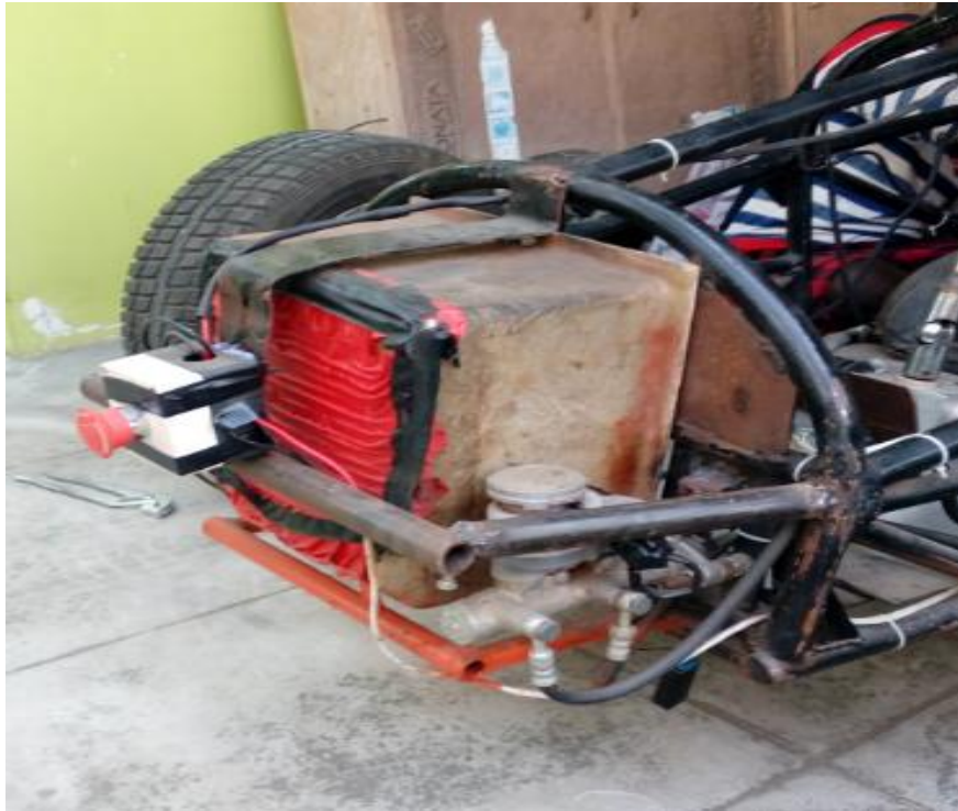
[Figure – 2.4.1 Impact attenuator]
