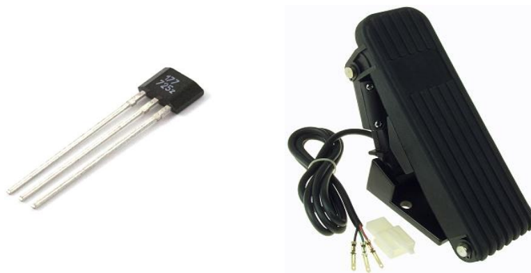
[Figure - 4.5 Hall effect sensor and Pedal in which hall sensor is incorporated]
