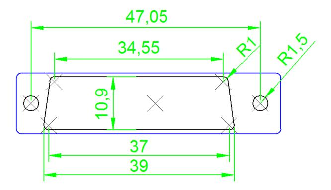
Hole for DB25F connector. Blue- external shield, black- hole , two round holes for screws.
