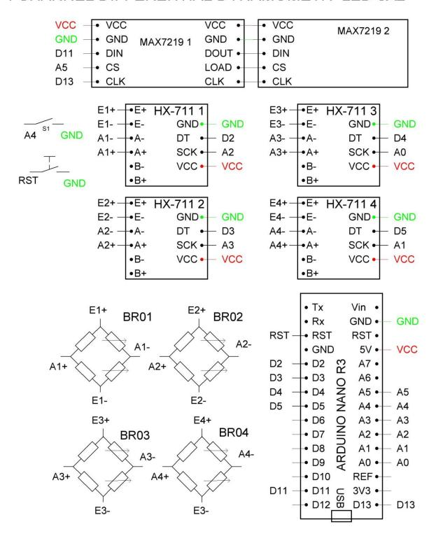
Power supply is over miniUSB connector of Arduino Nano. It is usefull to solder some 0.1 uF 16 V capacitors on GND and VCC junctions of HX-711 shields, and 3300 uF 16 V low ESR capacitor parallel to VCC and GND pins.
