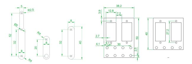
The size of components are defined by the servo in use. We made all drawings for Servo mini SG90 9g Tower Pro. Here is one block
