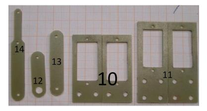
The only difficult part of mechanics component fabrication is lever arm 12. The perforation on arm must fit servo shaft perforation. We make perforation by drilling 20 holes via  $18^{\circ}$  (our servo shaft has 20 teeth) with 1mm radius drill with centers on the R=1.87 mm circle.
