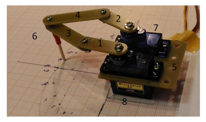
download ServoPot2Tester.ino program. We rotate potentiometers until the pointer is in the point we need. On monitor we can see the values of servo angles, we denote this angles as fi and psi.
