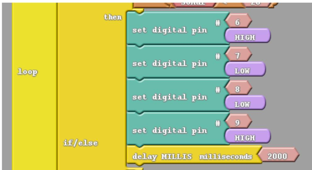
14. Snap another four "Set Digital Pin" panels into the "else" slot and set their values as shown.
