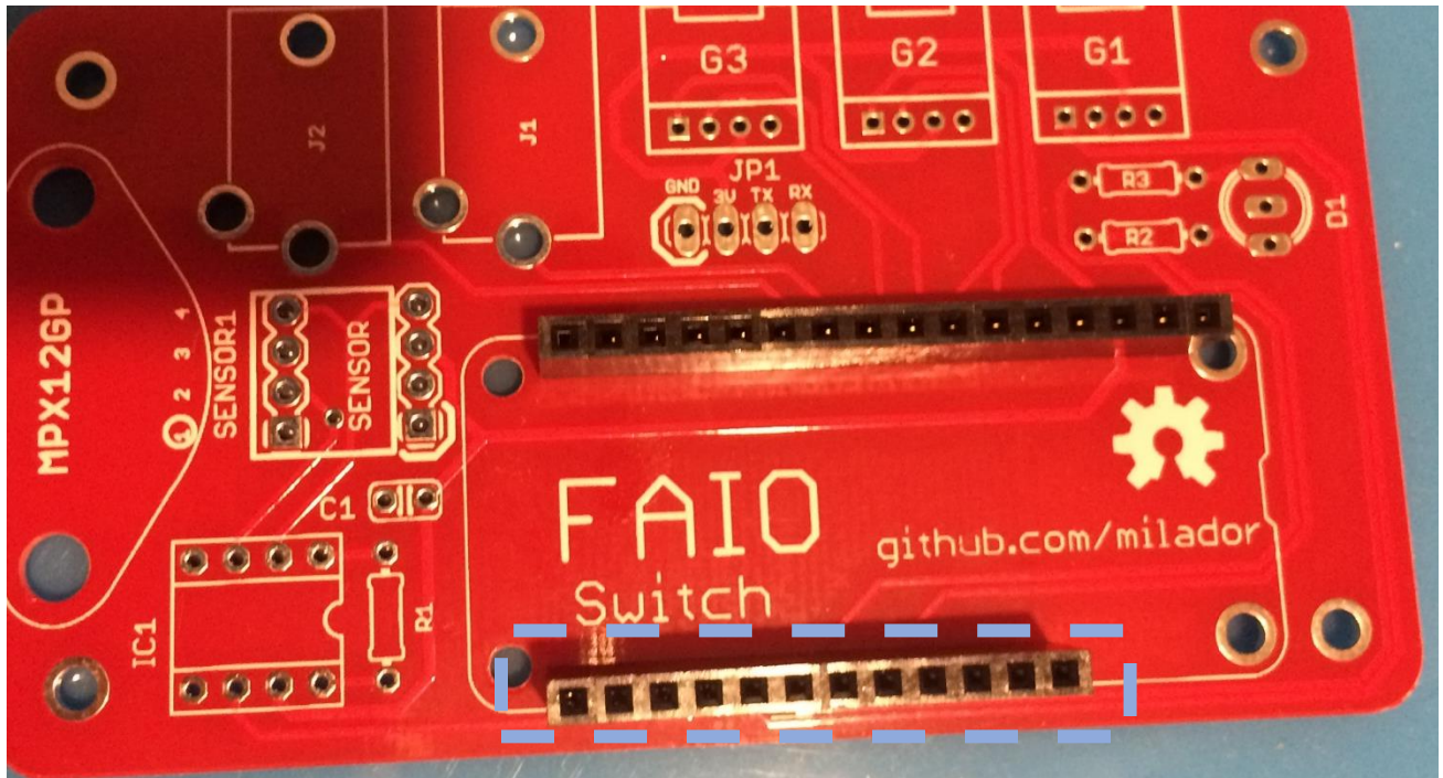
Step 5 – Solder 14 position female header connector
