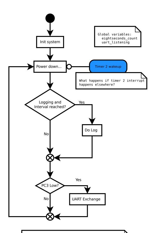
Actually the logger doesn't begin logging after power-up. It waits for logging setup via UART before doing anything. Inserting the battery doesn't start logging.
