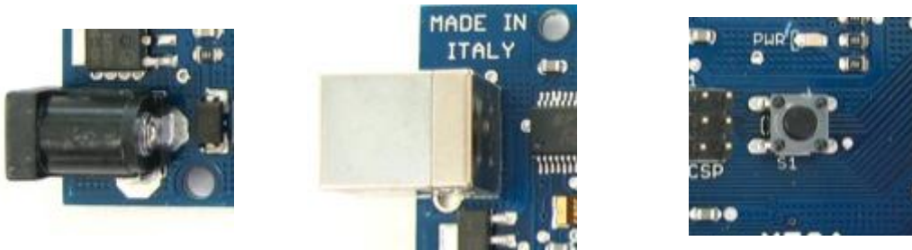
Figure 1: A) The 5mm barrel jack; B) The USB B female jack; C) The reset button.
