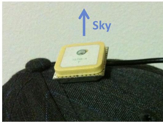
Figure 2: Correct placement of the GPS antenna.
