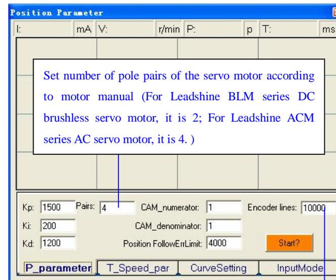
Set the Encoder Lines according to encoder specification. The input number should be 4 times of the actual encoder lines/resolution since the ACS806 decodes the encoder signals in X4 mode (ie. 10000 for 2500 lines encoder).
