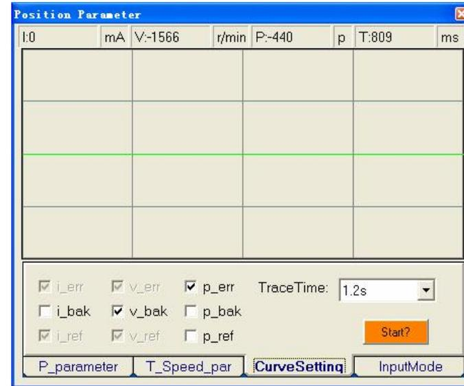
Figure 32: Digital Scope settings for the tuning
