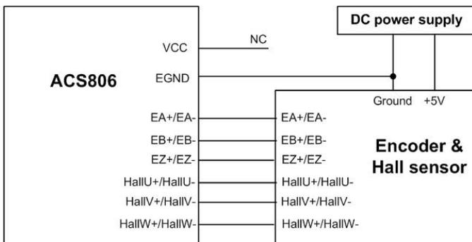
Figure 8: Using external DC power supply to supply the encoder
