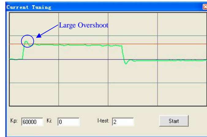
Figure 28: Response with High  $K_p$  of current-loop ( $K_p = 60000$ )
