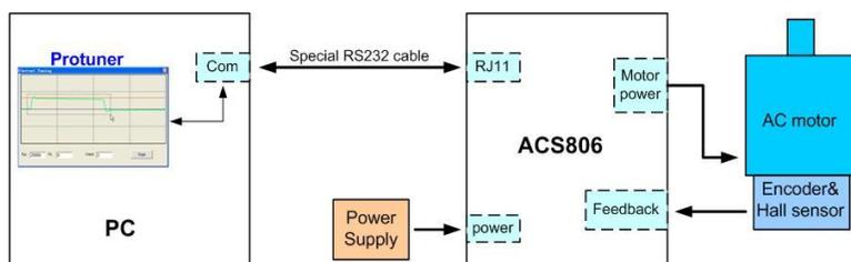
Figure 20: Configuration and connections before Tuning
