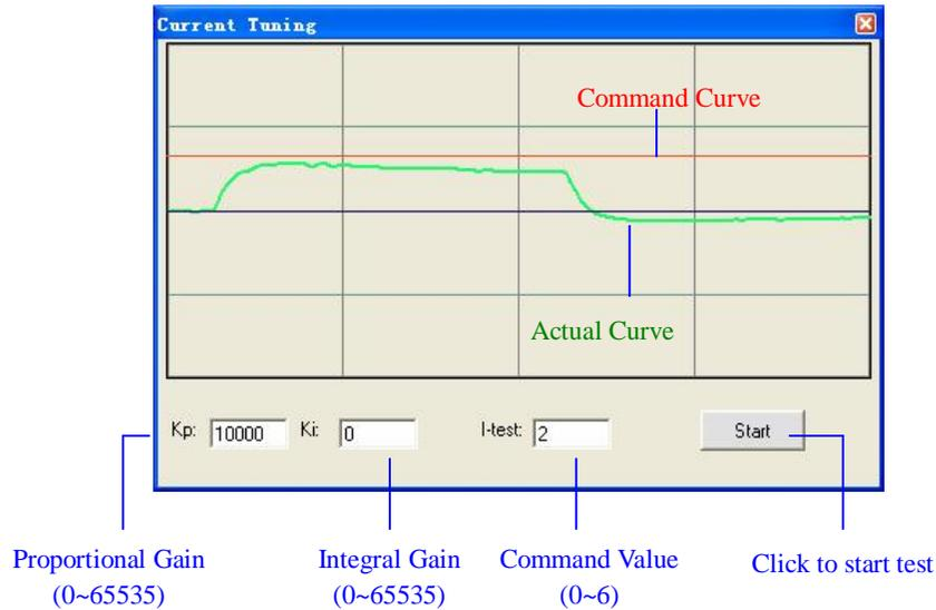
Figure 26: Current-loop tuning window
