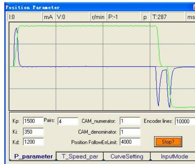
Figure 43: Position following error curve and velocity curve (Kp=1500, Ki=350 and Kd=1200)
