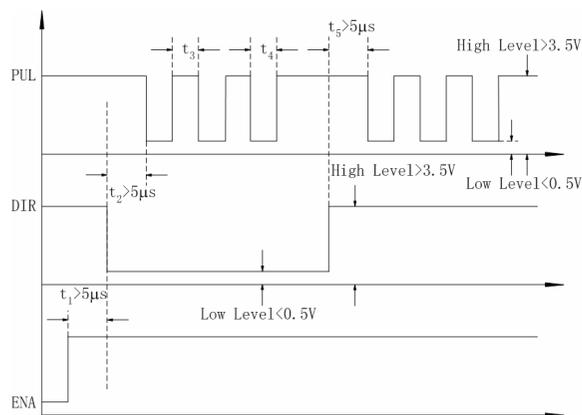
Figure51: Sequence chart of control signals
